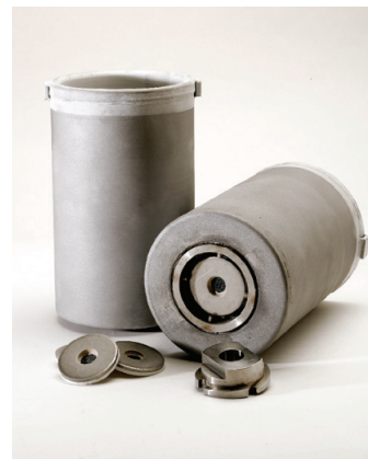
PoDFA reusable crucible and filter
