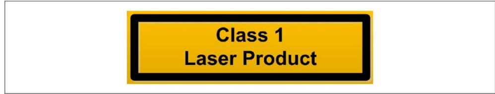
Meaning: Class I infrared laser beam invisible to the human eye.
