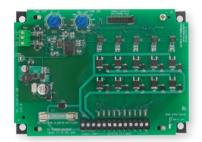
The SERIES DCT500ADC Low Cost Timer Controller is designed to provide continuous or on-demand cleaning for 10-35 volt powered receivers and pulse jet systems. It is available in either 4, 6, or 10 channels, and each unit is the same size, minimizing enclosure space and reducing overall system installation cost. For added safety, the control circuitry including the control inputs are isolated from the line voltage.
