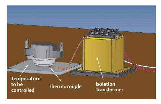
Figure 4 – Thermocouple placed externally to thermostat
