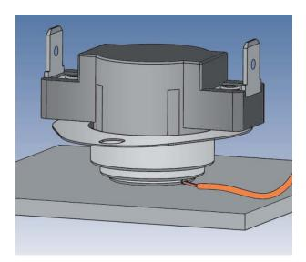
Figure 5 – Close-up of Thermocouple Placement
