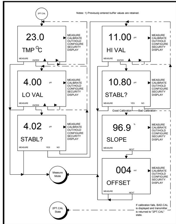
**Figure 13 – Screen Flow Diagram for Two-Point Process Calibration**
