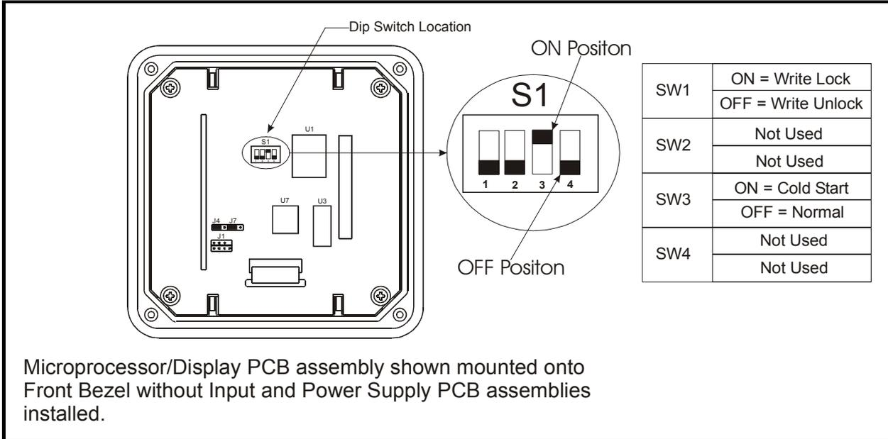
**Figure 33 – Hardware Dip Switch Location and Function**
