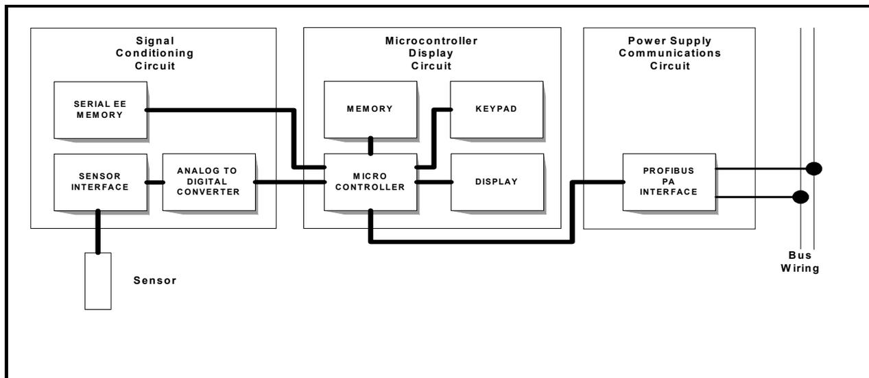
Figure 3 – Functional Block Diagram for TB82 PROFIBUS PA Transmitter
