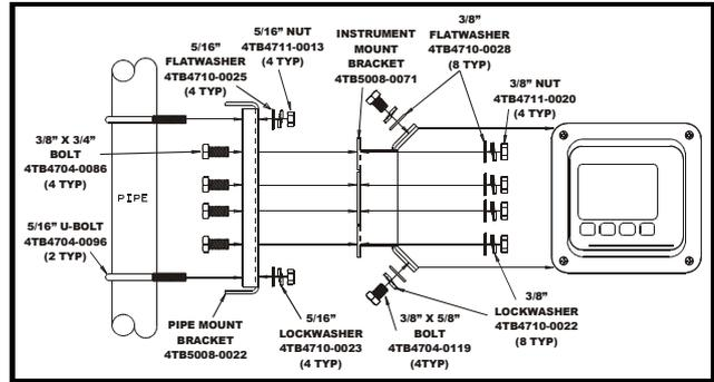
Figure 5 – Pipe Mounting Detail
