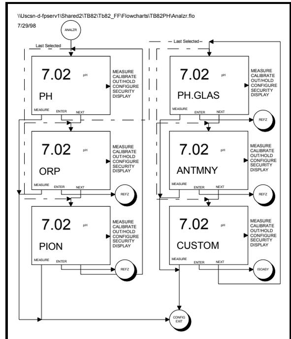
Figure 20 – Screen Flow Diagram for Analyzer and pH Analyzer States of Operation
