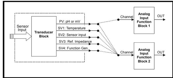
**Figure 32 - Possible Connections Between the TB and AI's**
