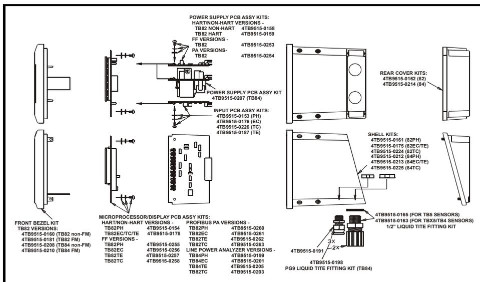
Figure 34 - TB82PH PROFIBUS PA Transmitter Exploded View
