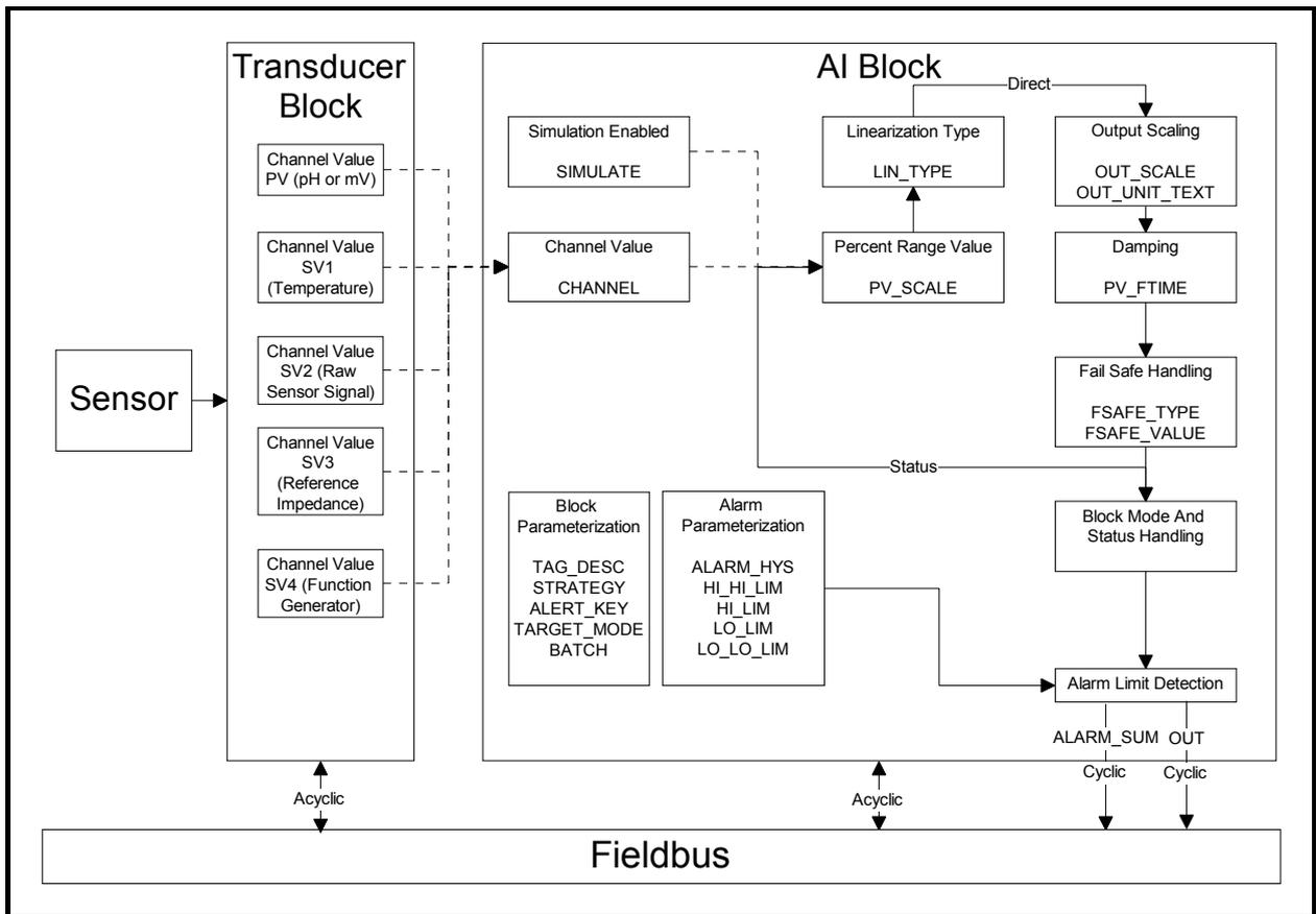
Figure 31 – Analog Input Two Function Block Design Diagram
