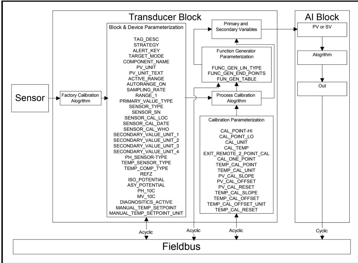
**Figure 29 – Transducer Block Design Diagram**
