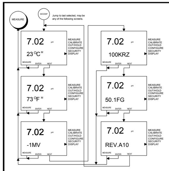
Figure 26 – Screen Flow Diagram for Secondary Display Mode of Operation
