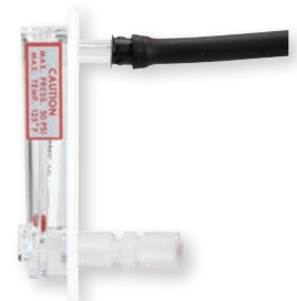
Model MMF connections. Connector at top, installed in panel, has retainer and flexible tubing in place. Connector at bottom shows alternative connection with metal or rigid plastic tubing, using a double compression nylon tube union (as Dwyer Part No. A-328).
