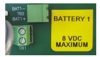
Figure 6. Power Connectors for Solar Panel and Battery 1
