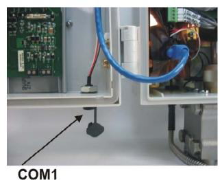
Figure 5. COM1 Connector (in Door) for Local Communication Access
