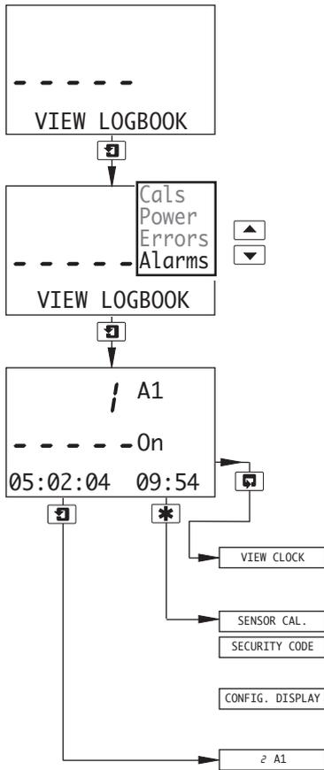
The logbook stores data entries for alarm events, sensor errors, power failures and sensor calibrations.
