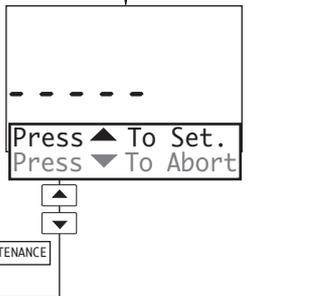
**Press ▲ to Set** and **Press ▼ to Abort** are displayed alternately on the lower display line.
