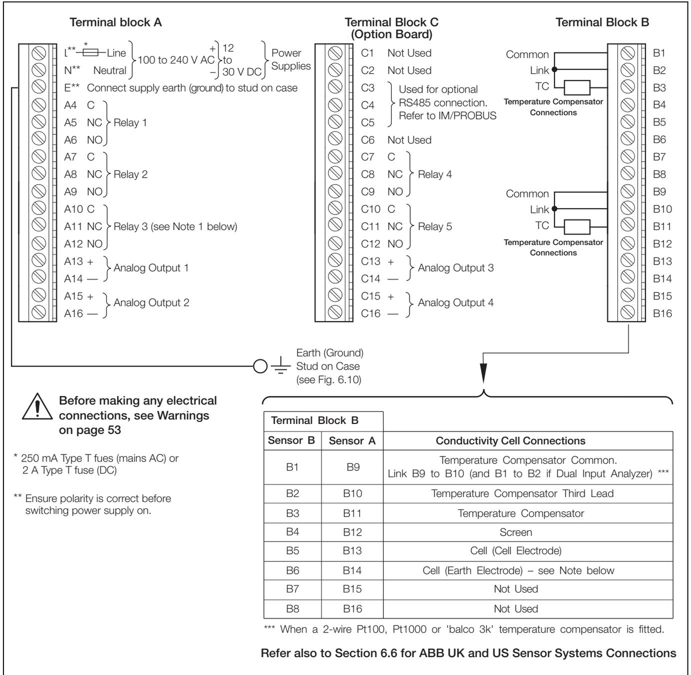
Fig. 6.11 Connections, Panel-mount Analyzers
