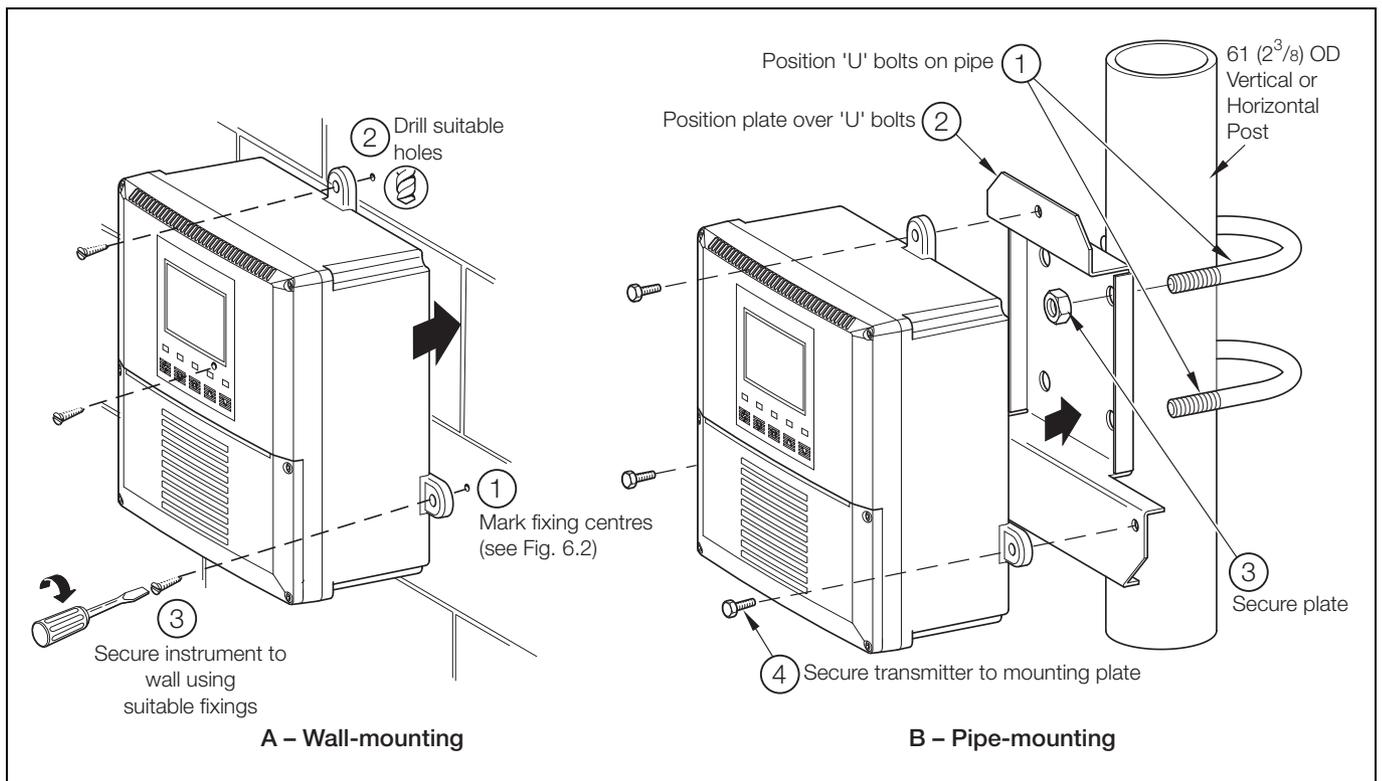
Fig. 6.3 Wall-/Pipe-mounting
