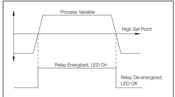
Fig. 5.4 High Non-Failsafe Alarm without Delay and Hysteresis
