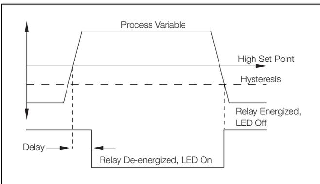
Fig. 5.3 High Failsafe Alarm with Hysteresis and Delay
