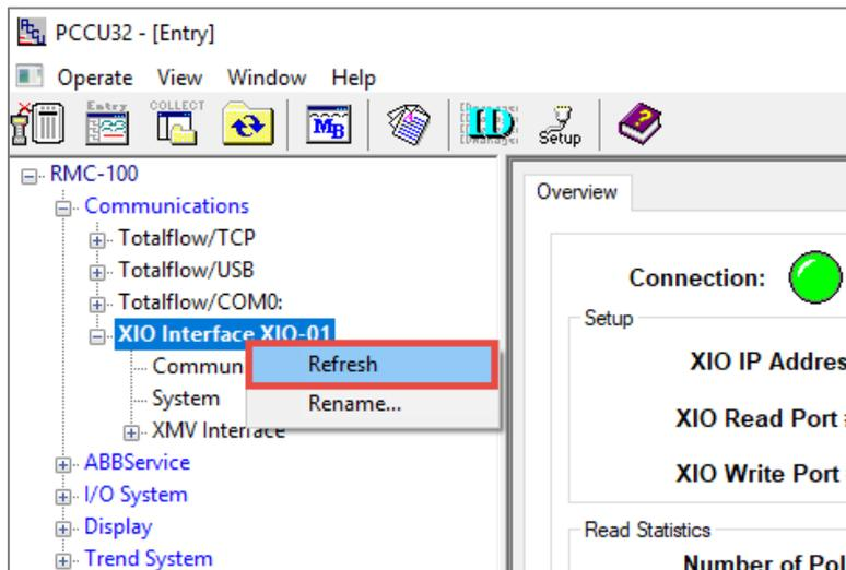
2. On the navigation tree, expand the XIO Interface instance to display all its detected applications.
