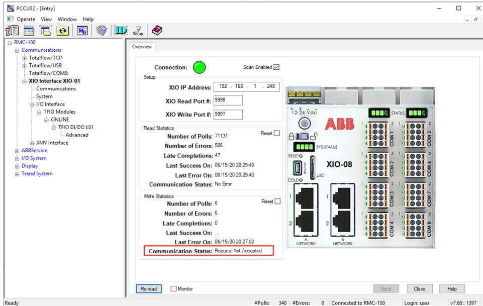
**Figure 5-3: Write Communication Status error message - Request Not Accepted (Setup)**
