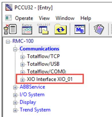
12. If unable to see the XIO interface on the navigation tree, refresh the navigation tree or click **Close**. View or reconnect to verify the navigation tree displays the XIO Interface application.
