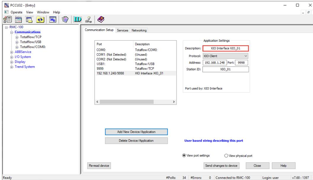
11. Click **Send changes to device**. The XIO Interface application displays in the navigation tree (Figure 2-4).
