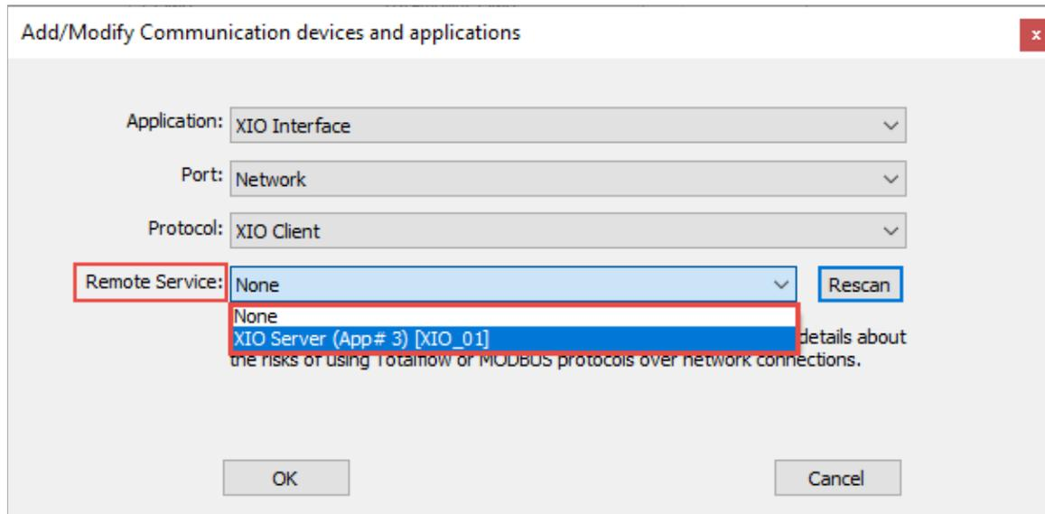
When the RMC detects an XIO, it automatically determines its unique Station ID, IP configuration and XIO server TCP port information. These parameters are required to establish connection successfully.
