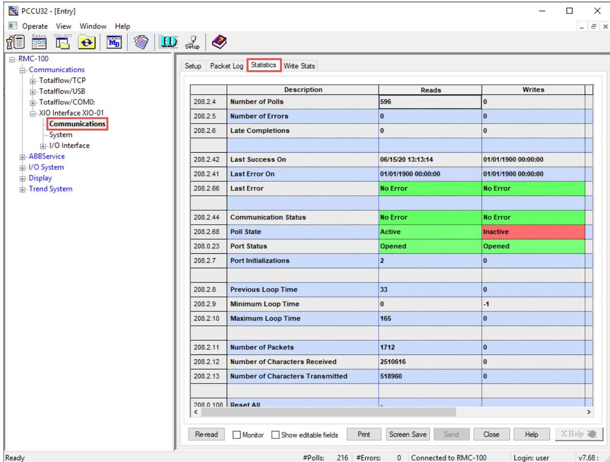
If an unusually high number of errors display, check communication parameter configuration on the Setup tab. Ensure parameter values, such as the XIO Station ID, IP address or TCP ports, match those on the XIO. Ensure that the security code that allows read/write access to the XIO is configured in the XIO Interface setup. The remote controller cannot perform reads or writes unless it has this code.
