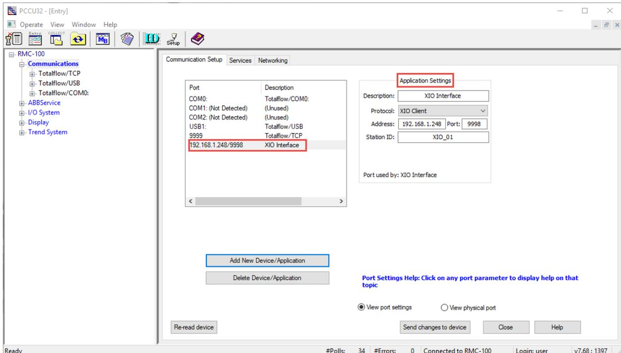
9. Verify the values of the additional configuration fields. The Application Settings section displays the generic description of the XIO Interface, default protocol, detected TCP parameters and XIO Station ID. These values are automatically populated when the XIO Interface was added.
