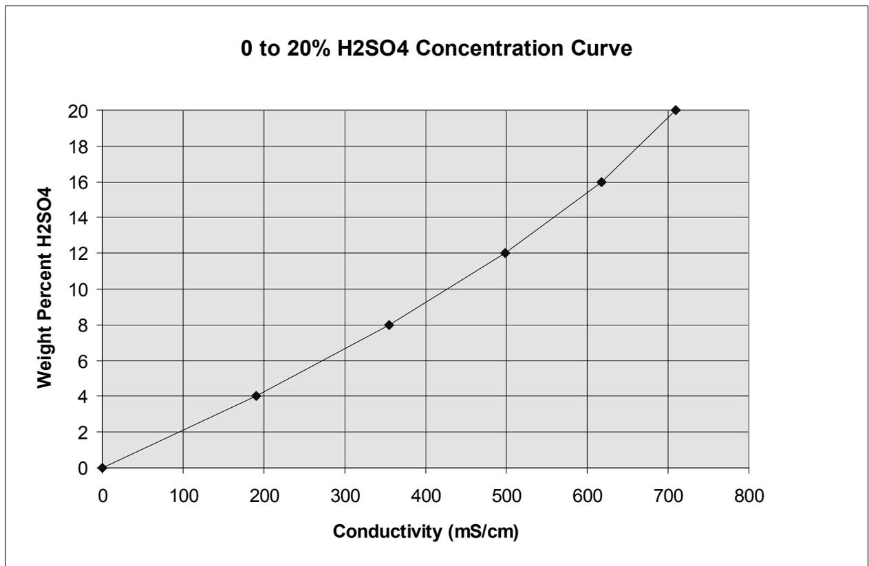
Figure B-4. 0 to 20% H<sub>2</sub>SO<sub>4</sub> Concentration Curve
