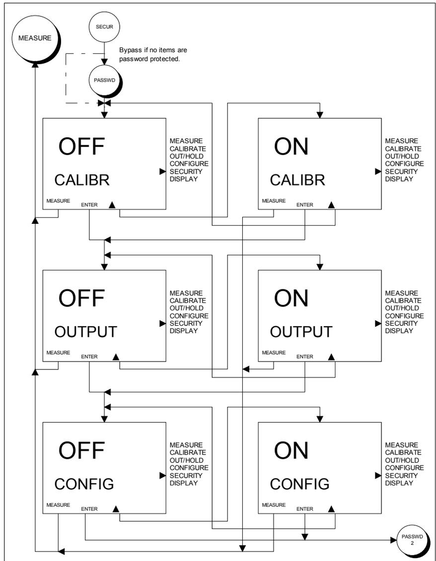
Figure 9-1. Screen Flow Diagram For Security State of Operation
