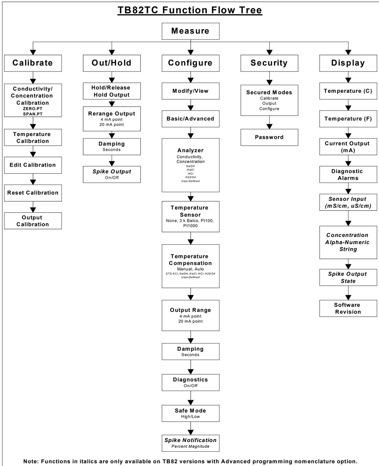
Figure C-1. TB82TC Programming Function Flow Chart.
