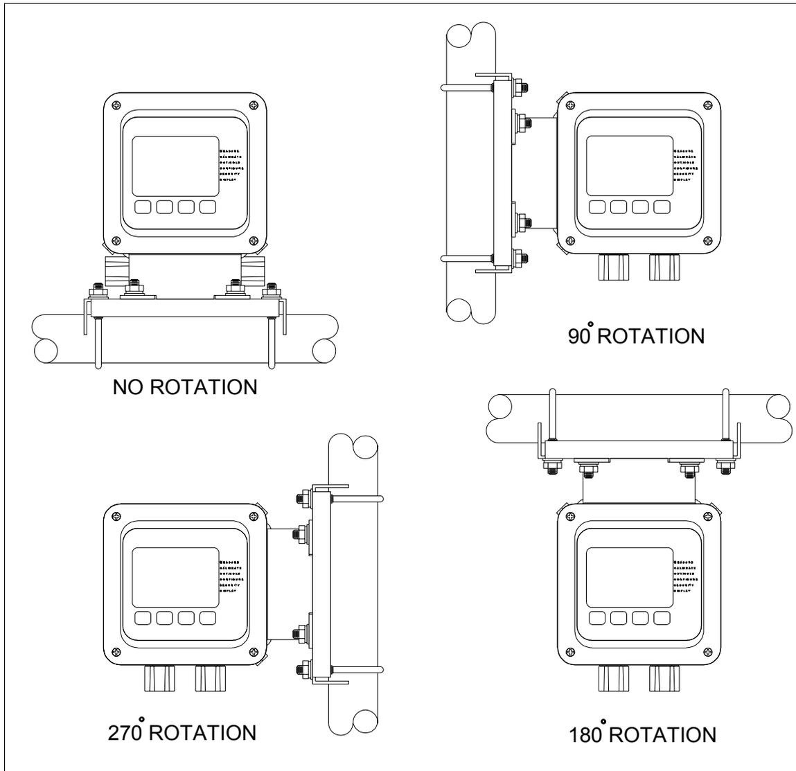
Figure 3-7. Mounting Rotation (Pipe Mount Shown)
