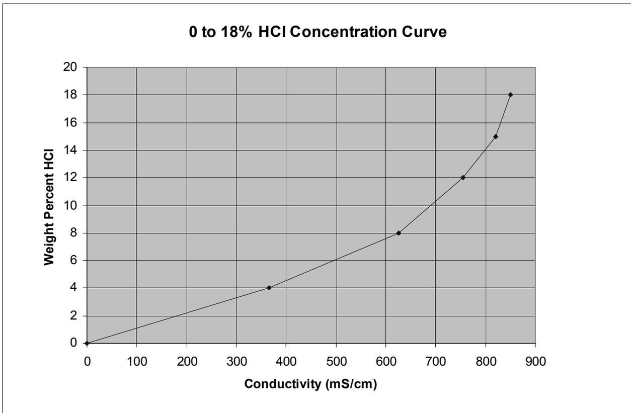
Figure B-3. 0 to 18% HCl Concentration Curve
