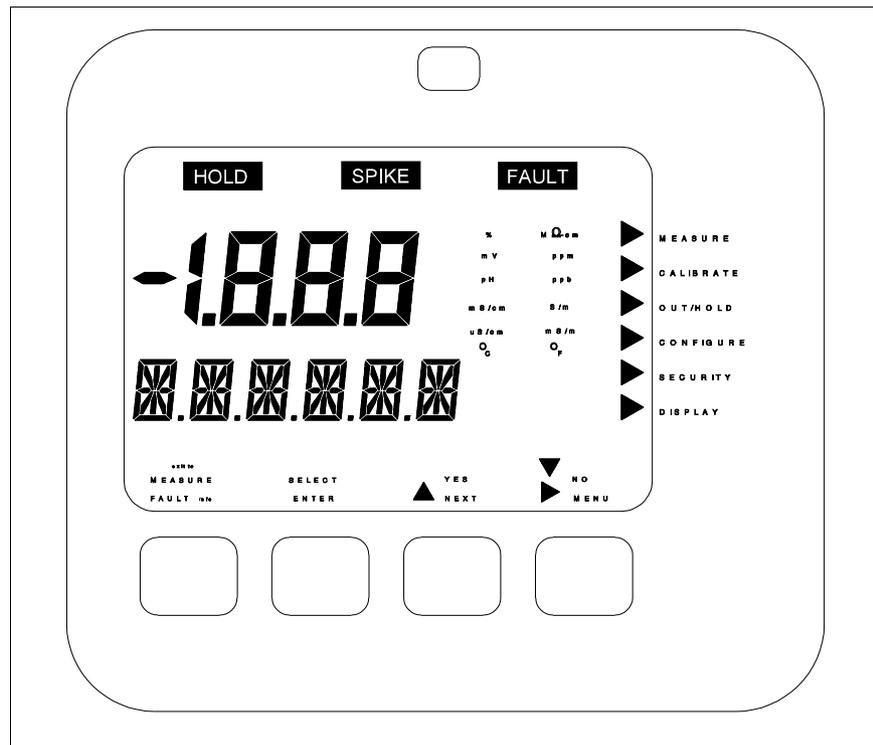
Figure 4-1. Fully Energized Display And Supporting Information
