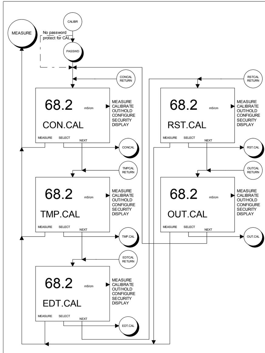
Figure 6-1. Screen Flow Diagrams For Calibrate States of Operation
