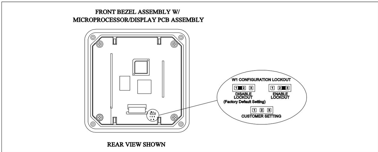
Figure 8-5. Configuration Lockout Jumper Location On Microprocessor/Display PCB Assembly.
