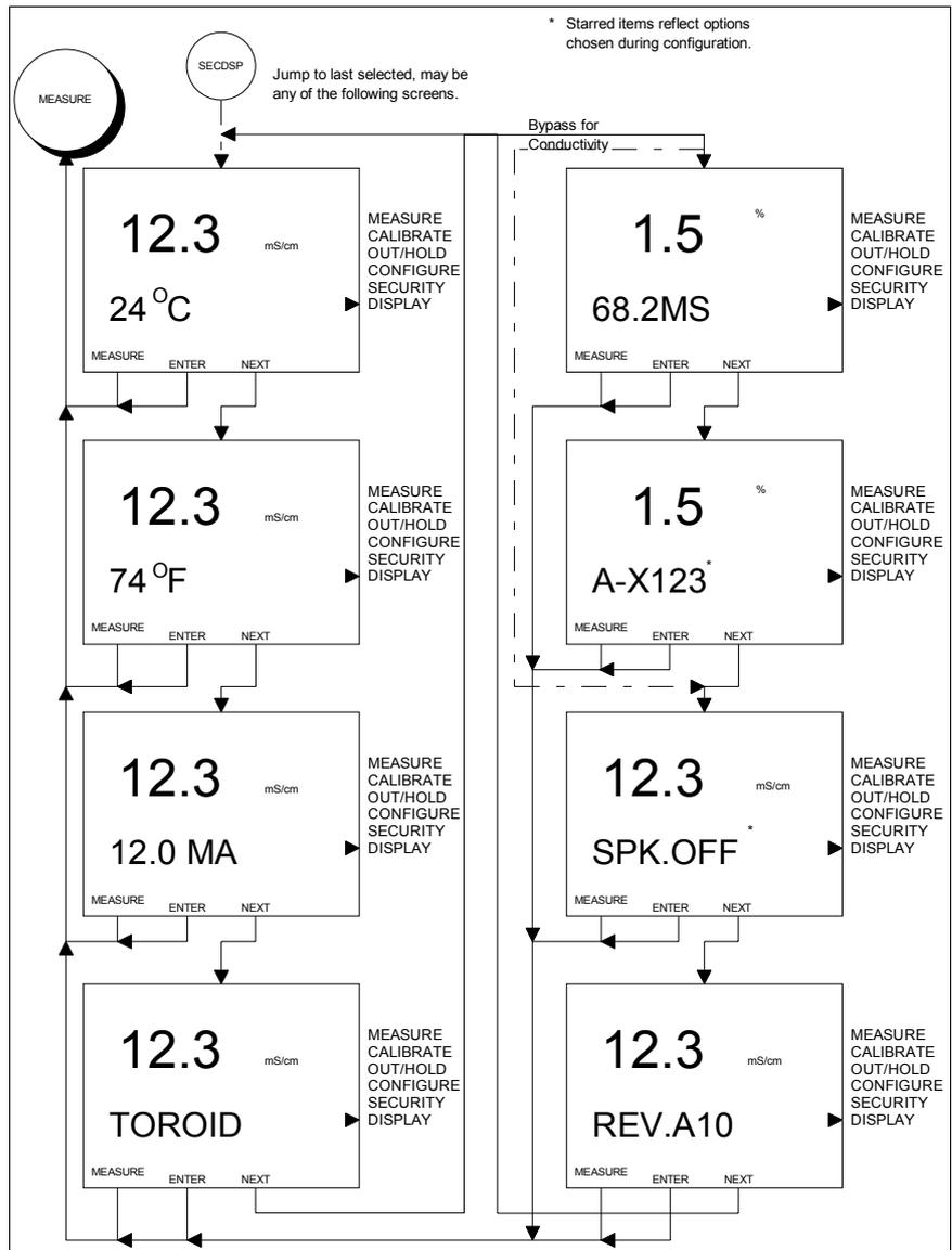
Figure 10-1. Screen Flow Diagrams For Secondary Display States of Operation.
