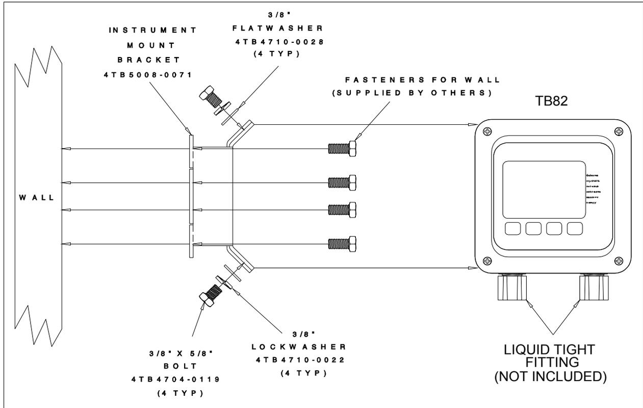
Figure 3-4. Wall Mount Installation Diagram
