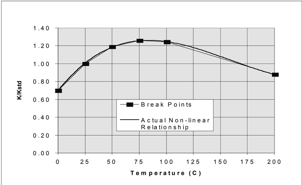
Figure 8-4. User-Defined Temperature Compensation Break Point Determination.
