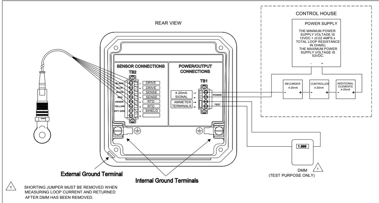
Figure 3-6. Instrument Wiring Diagram
