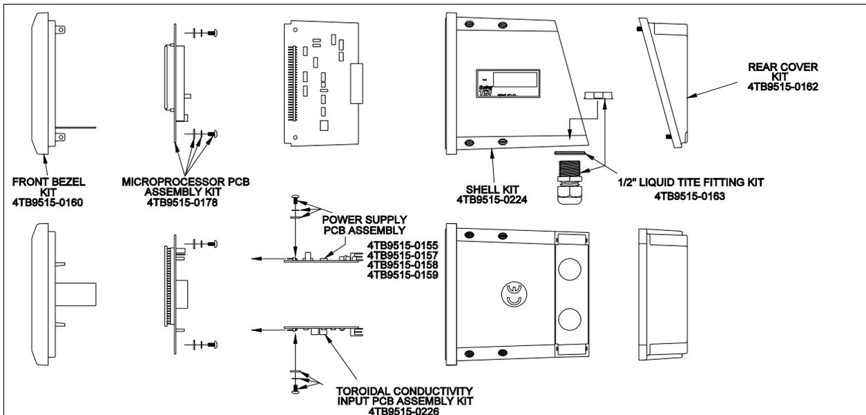
Figure 15-1. TB82 Advantage Series Exploded View Showing Kit Assignments.
