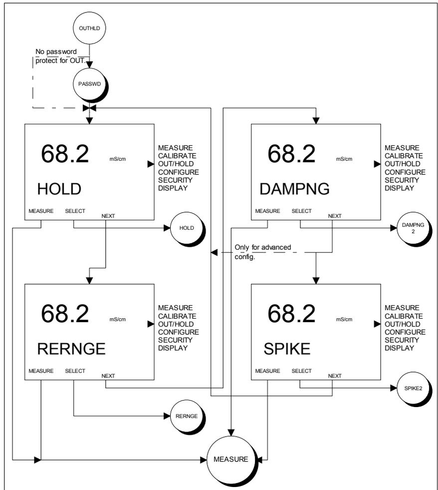
Figure 7-1. Screen Flow Diagrams For Output/Hold States of Operation
