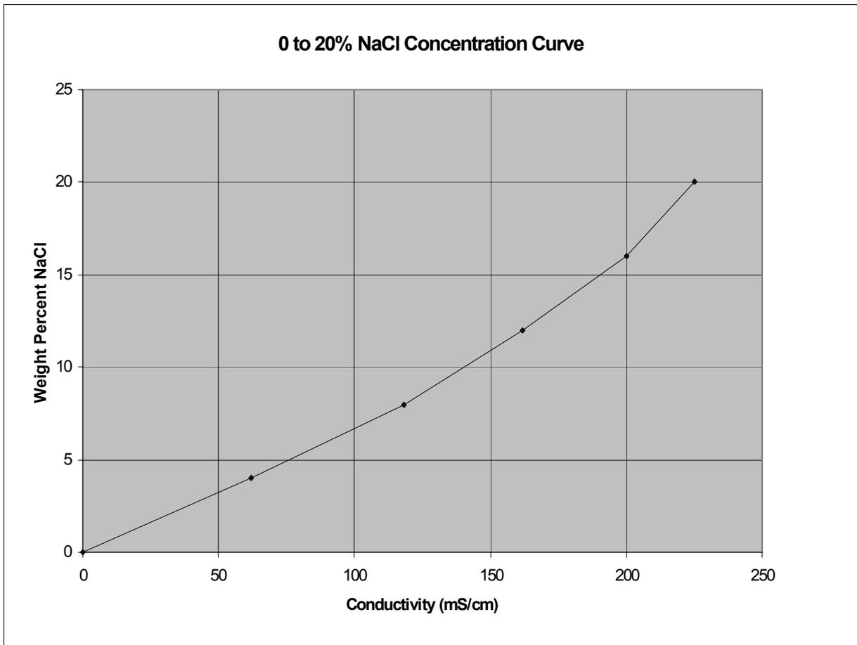
Figure B-2. 0 to 20% NaCl Concentration Curve
