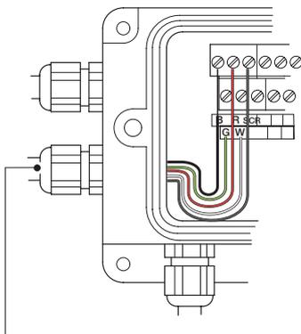
**Additional serial cable connections to multiple wet-sections**
