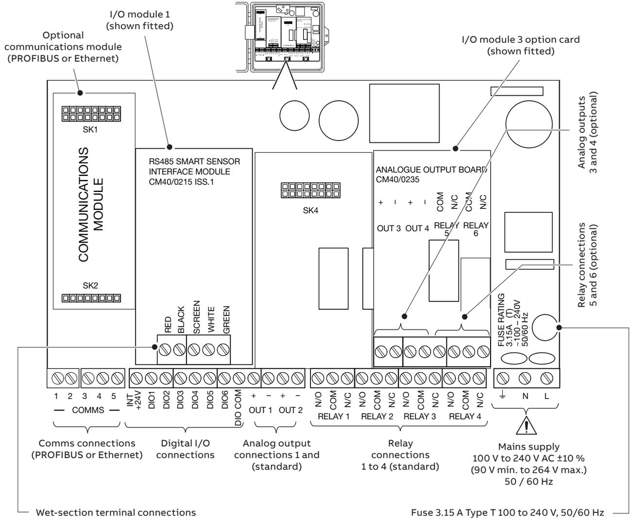
**Digital I/O, relays and analog output**
