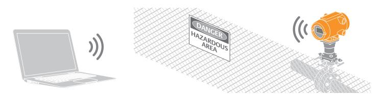
Secure Mobile SCADA allows local connection to the Flow Computer from a designated safe area for monitoring, data collection and configuration.
