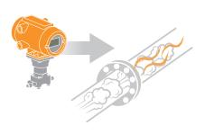
Odorizers and samplers can be driven directly from the flow computer's pulse outputs.
