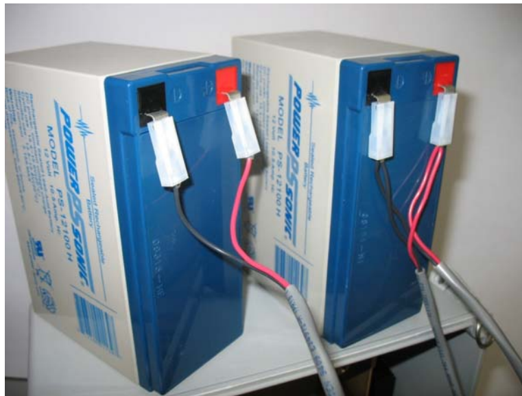
Figure 5-12: Connect New Battery – Both Now Connected
