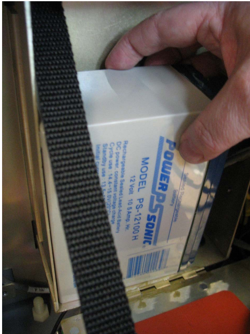
Figure 5-8: Pry Out the Old Battery Pack – Leave Connected to Cable
