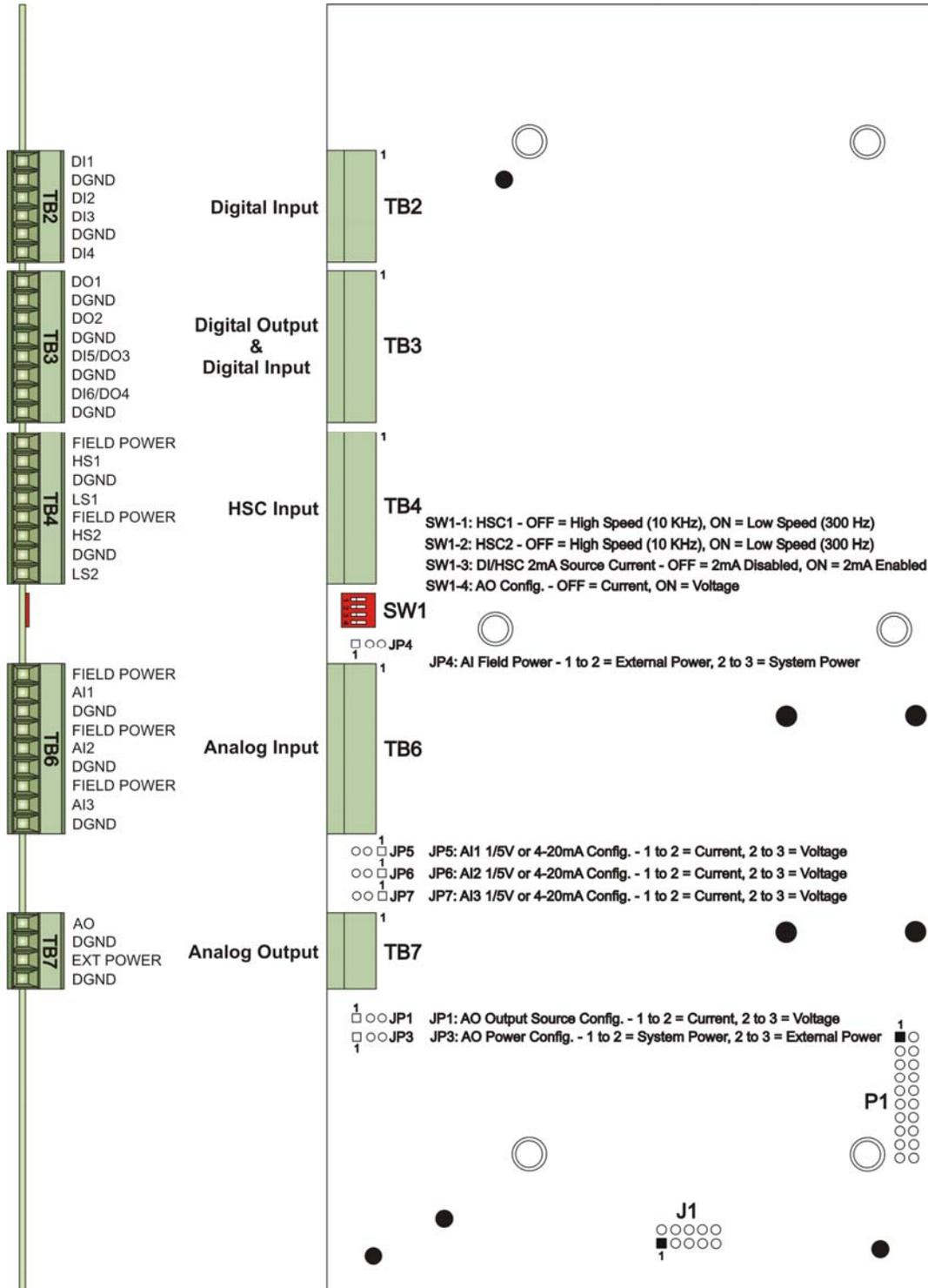
Figure 3-1. Process I/O Board Component Identification Diagram
