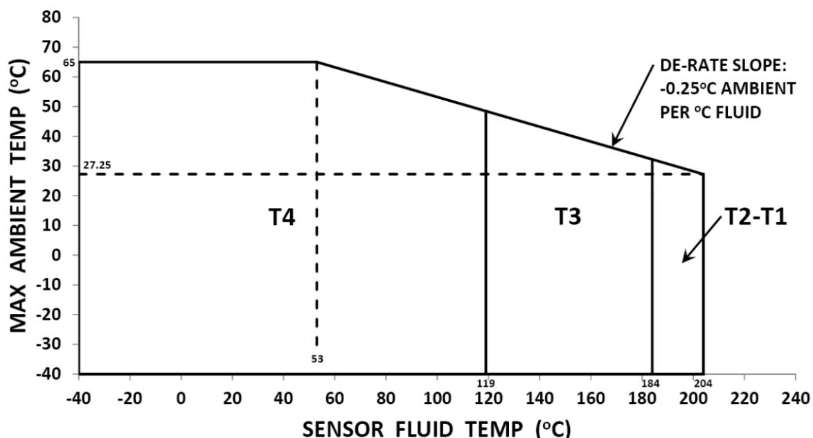
Note 1: Use the above graph to determine the temperature class for a given fluid and ambient temperature.
