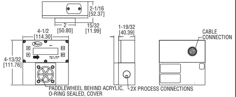
The **SERIES DPW** Digital Paddlewheel is an economical choice for applications where remote or local liquid flow measurement is desired. This Series offers two programmable totalizers via the optional LCD and RS-232/RS-485 interface, two optically isolated flow pulse outputs, and selectable 0 to 5 VDC or 4 to 20 mA flow outputs (optional temperature).
