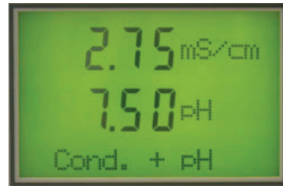
Simultaneous conductivity and pH measurement
