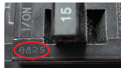
Example: Miniature Circuit Breaker HOM115CAFI (stamped near handle of device) 0825 = 2008, week 25 (June 16–22). There is no specific number listed for the day of the week.
