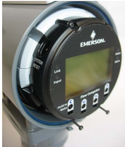
Figure 4-5: Removing the Battery Pack
