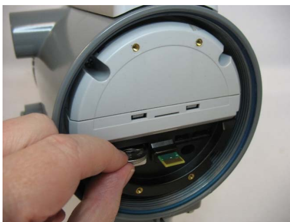
Figure 4-6: Removing/Replacing the Coin Cell Battery
