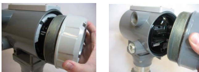
Figure 2-8: Front (left) and Rear (right) End Caps Removal
