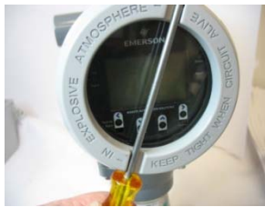
Figure 2-6: Removing or Tightening the End Cap with Long Screwdriver
