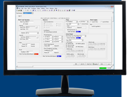
Action Blocks have five main sections: Block Logic Operation, Bypasses, Chain, Action Output, and Alarm Logging.
