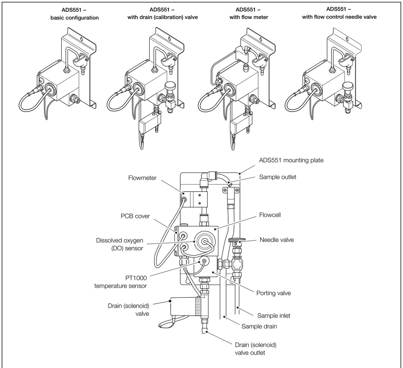
Fig. 2.3 ADS 551 low level dissolved oxygen wet-section – configuration options
