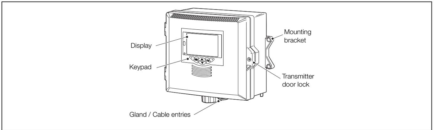
Fig. 2.1 Navigator 540 transmitter – main components
