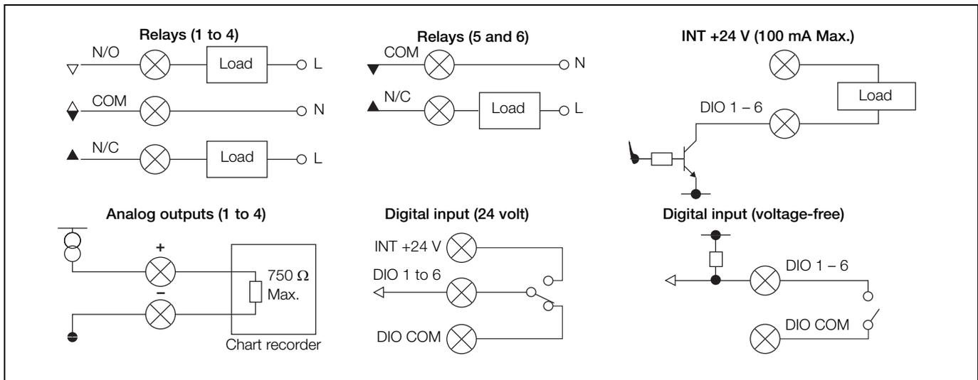
Fig. 3.18 Digital I/O, relays and analog output connections
