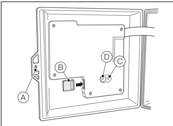
Fig. 6.12 SD card / USB stick insertion and removal
