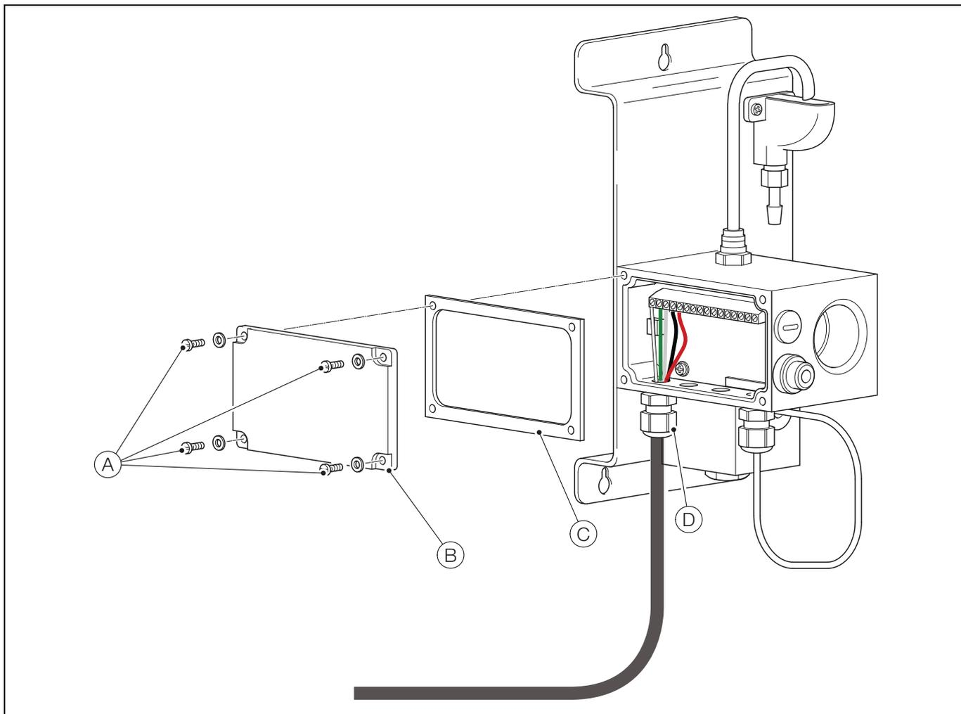
Fig. 3.14 Accessing the wet-section PCB – ADS551
