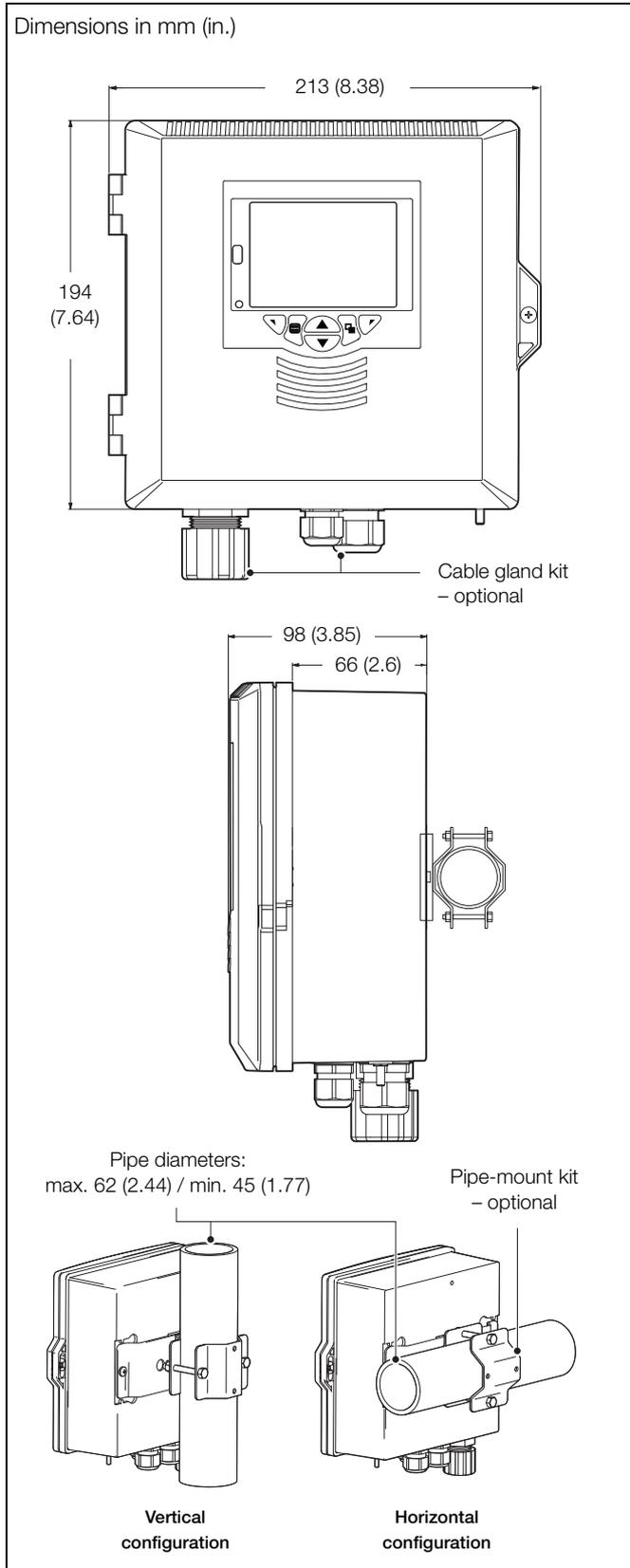
Fig. 3.9 Transmitter pipe-mount options
