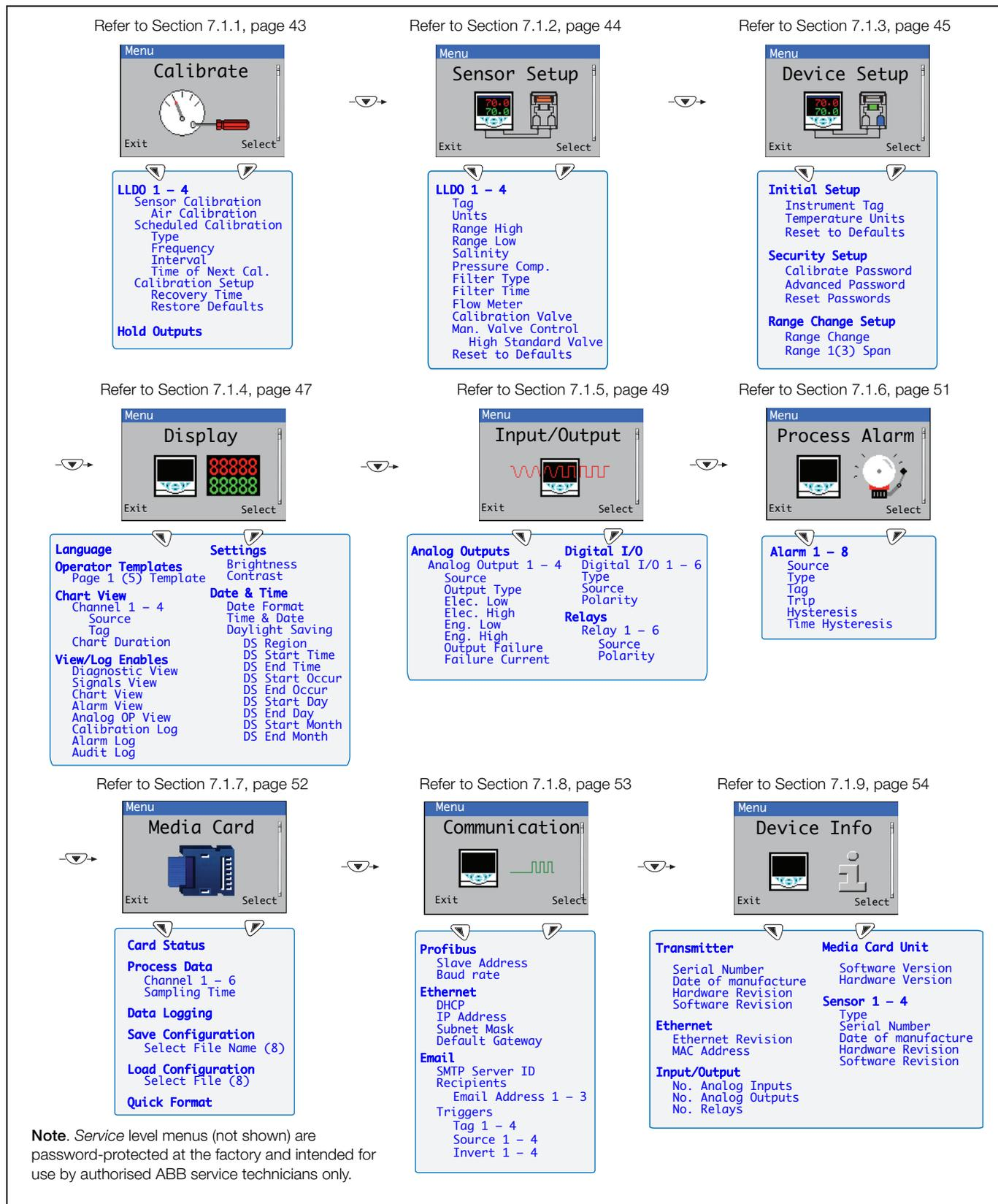
Fig. 7.1 Overview of low level dissolved oxygen menus
