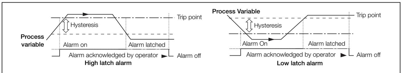
Fig. 7.3 High and low latch alarm action
