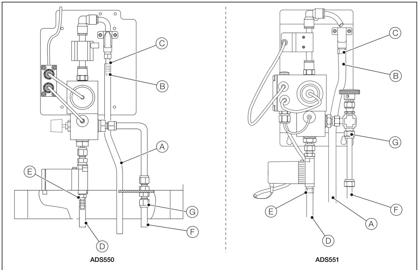
Fig. 3.6 Connecting the sample lines
