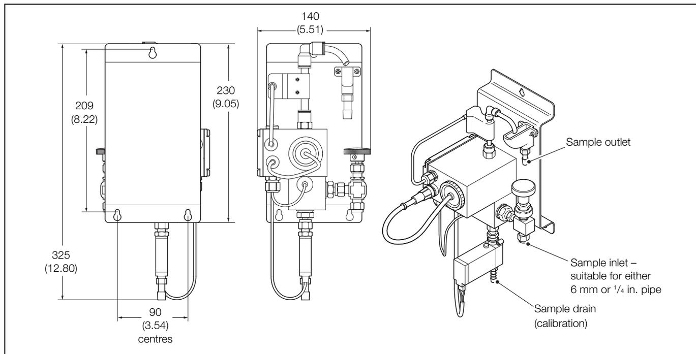
Fig. 3.4 ADS551 wet-section / mounting panel dimensions
