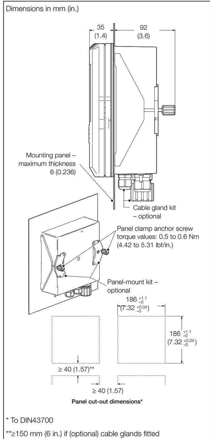
Fig. 3.8 Transmitter panel-mount option
