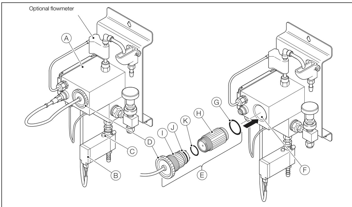
Fig. 8.2 Cleaning / Changing the dissolved oxygen sensor – ADS551
