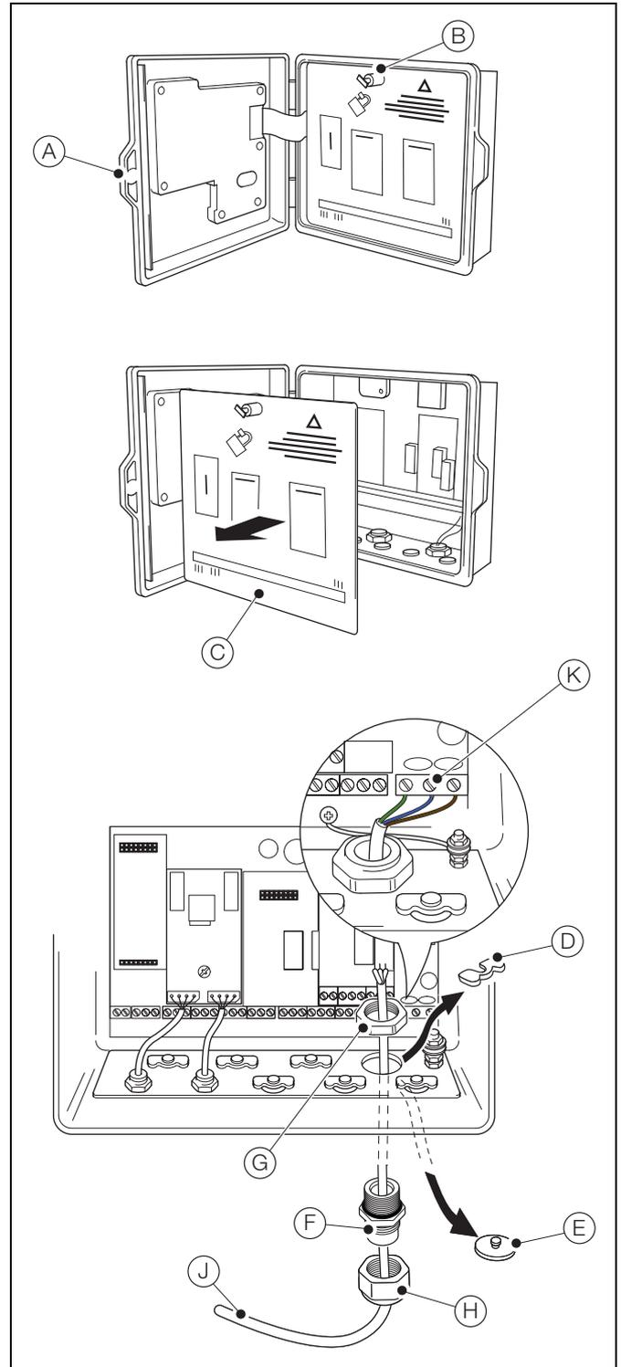
Fig. 3.16 Accessing the transmitter board and making electrical connections
