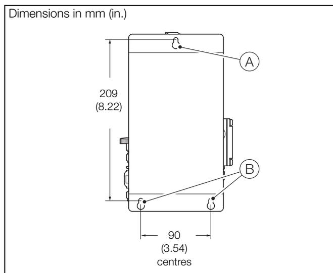
Fig. 3.5 Mounting the ADS551 wet-section panel
