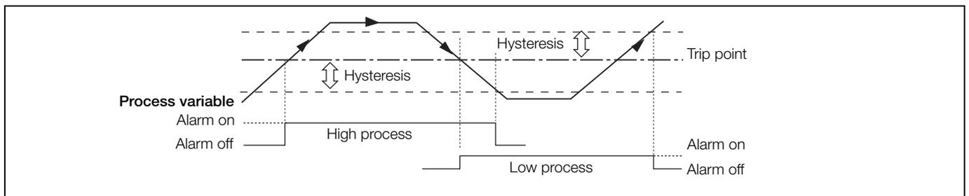
Fig. 7.2 High and low process alarm action
