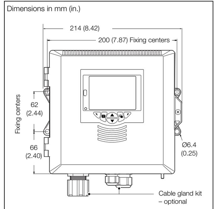
Fig. 3.10 Transmitter wall-mount option
