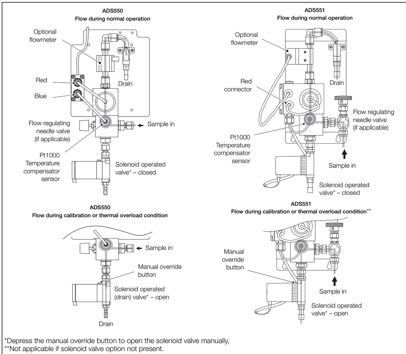
\*Depress the manual override button to open the solenoid valve manually,
