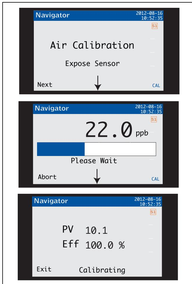
Fig. 5.2 Calibration procedure (without calibration valve fitted)
