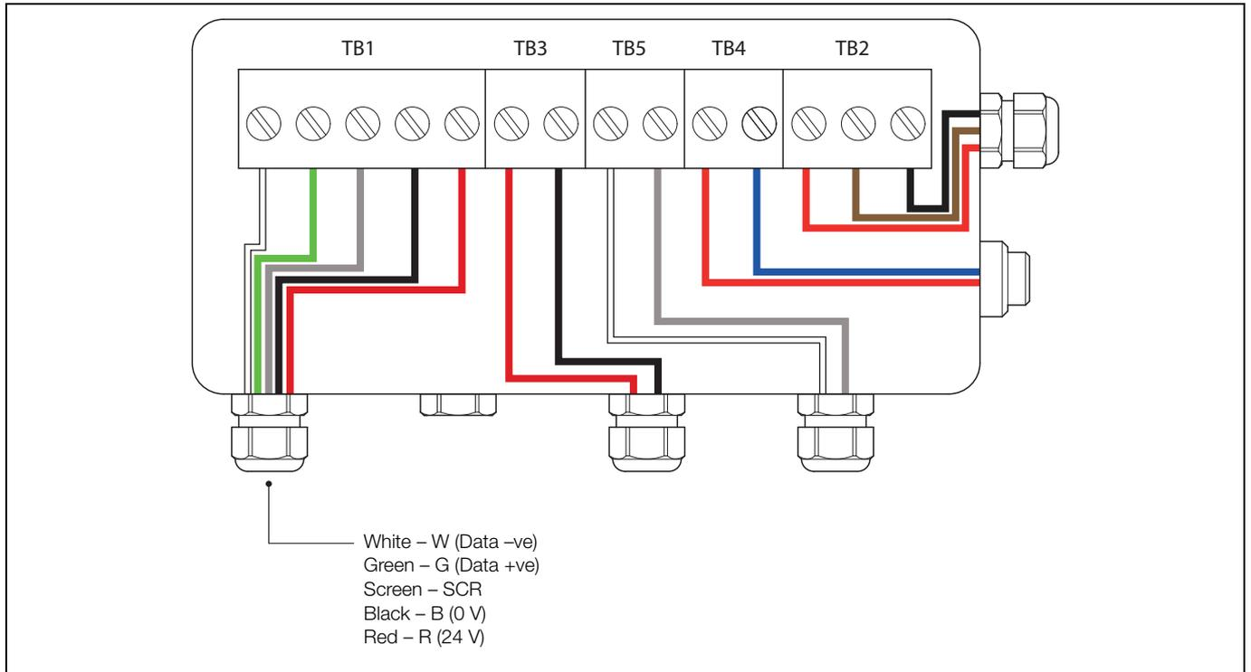
Fig. 3.15 Additional serial cable connections to multiple wet-sections – ADS551
