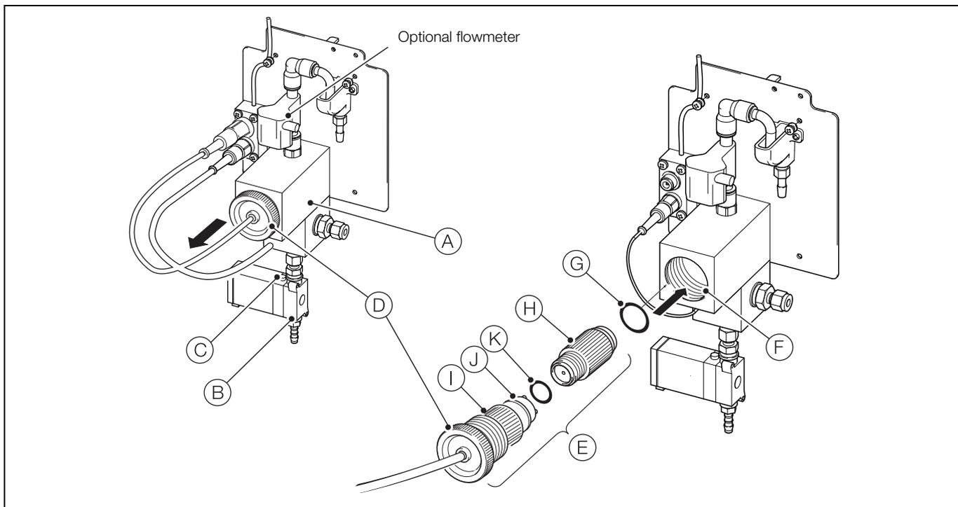
Fig. 8.1 Cleaning / Changing the dissolved oxygen sensor – ADS550
