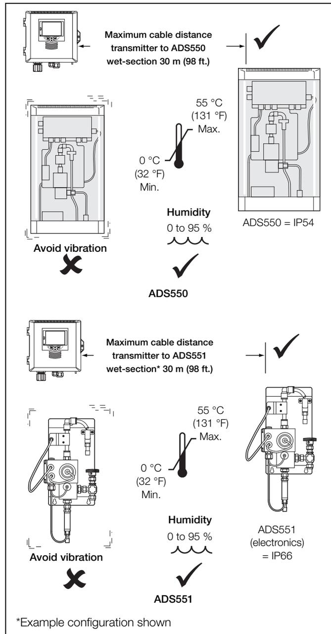
Fig. 3.1 Locating the wet-section
