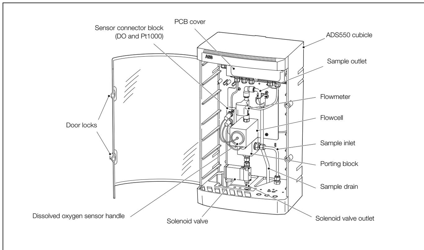
Fig. 2.2 ADS550 low level dissolved oxygen wet-section – main components
