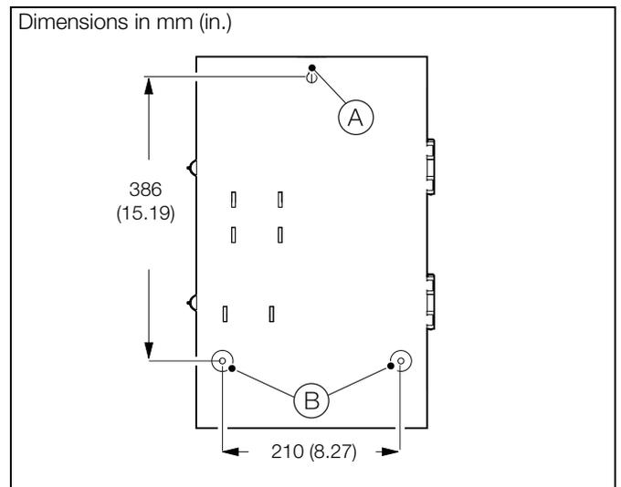
Fig. 3.3 Mounting the ADS550 wet-section cubicle
