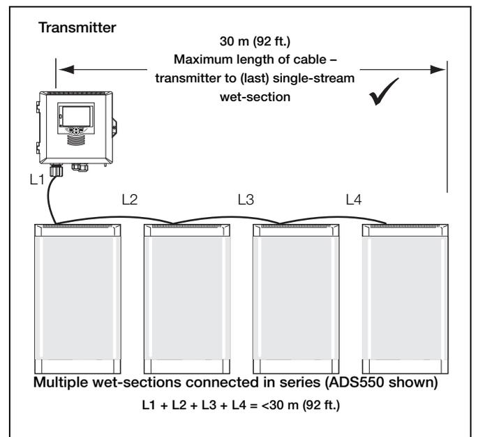
Fig. 3.11 Multiple wet-section setup – maximum cable length
