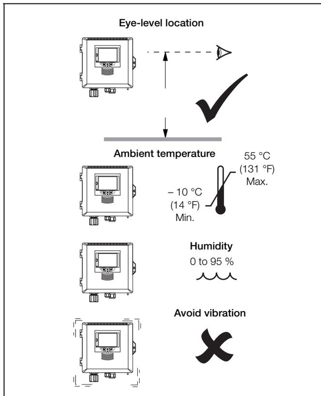
Fig. 3.7 Transmitter location
