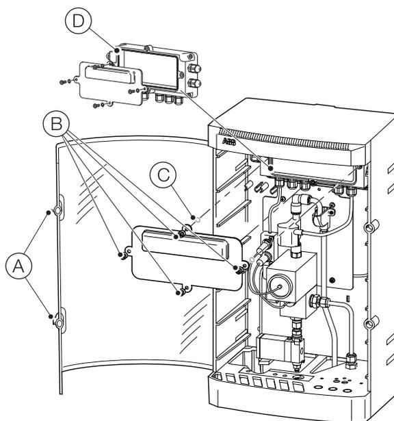
Fig. 3.12 Accessing the wet-section PCB
