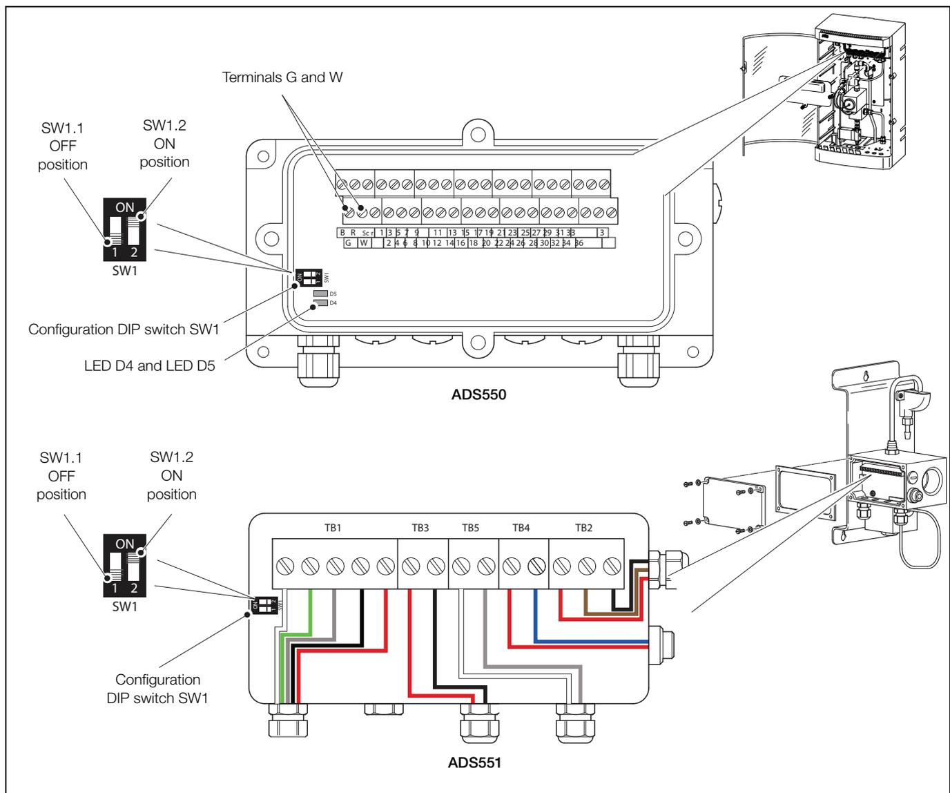
Fig. B.1 Configuration DIP switch SW1 (ADS550/ 551) and LED D4 / D5 location (ADS550)
