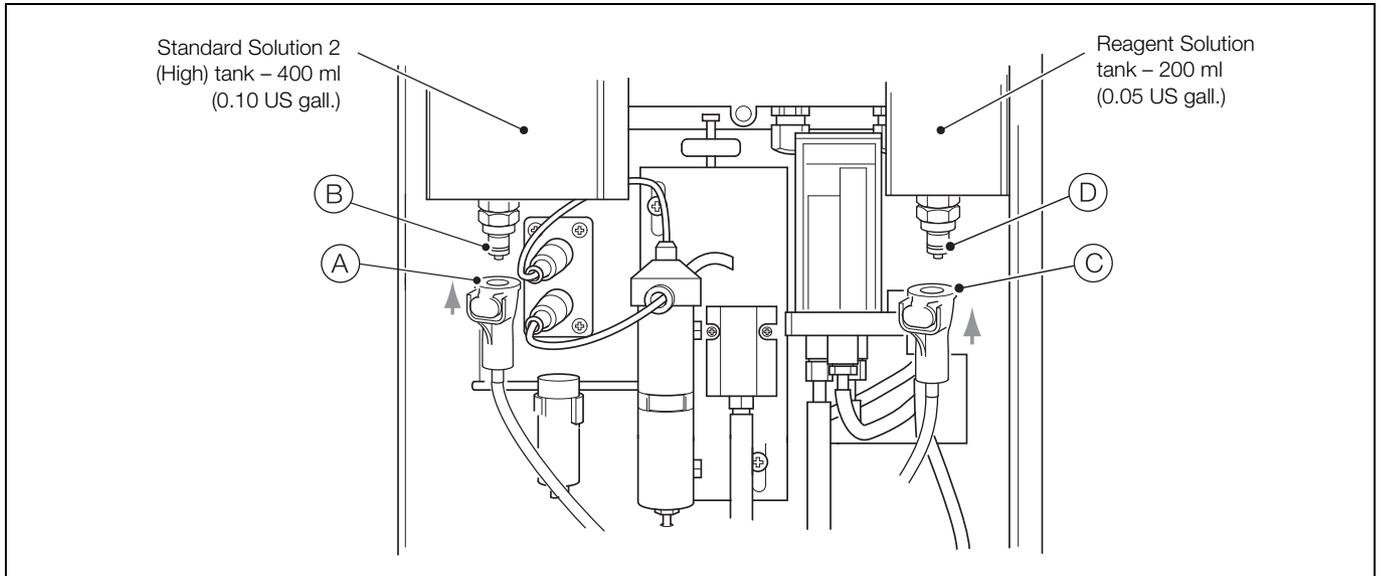
Fig. 3.5 Standard solution 2 (high) and reagent tubing connections
