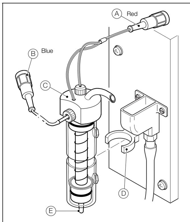
Fig. 8.4 Hydrazine sensor removal
