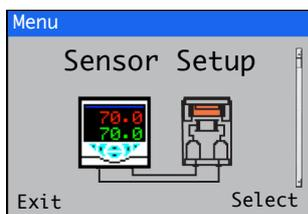
Used to set the wet-section tag, measurement units, operational range and filter type, enable / disable the *Flow Meter* (optional) and energize the solenoid valve (via the *Man./ Valve Control* menu).
