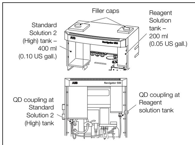
Fig. 8.1 Solution tanks
