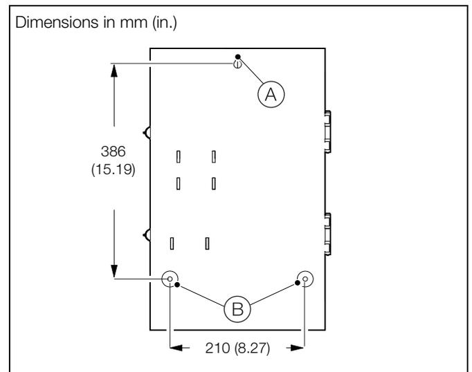
Fig. 3.3 Mounting the wet-section
