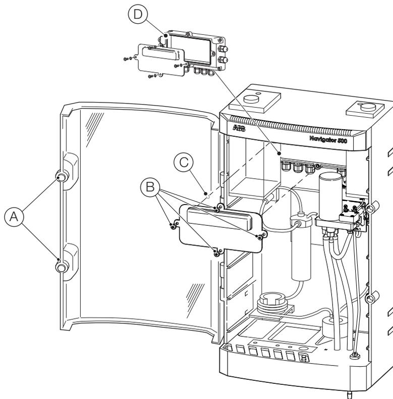
Fig. 3.11 Accessing the wet-section PCB
