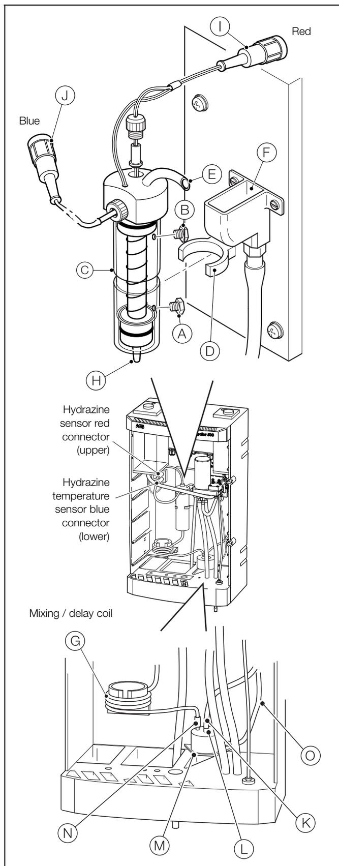
Fig. 4.1 Setting up the sample flow
