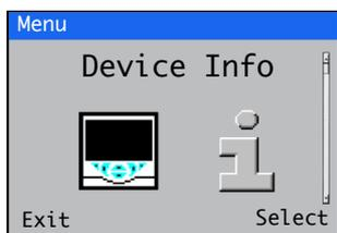
Displays read-only factory-set details for the transmitter and connected wet-section(s).
