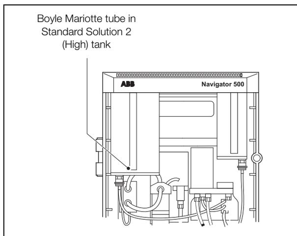
Fig. A.1 Boyle Mariotte tube in standard solution 2 (high) tank
