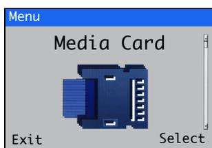
Used to set the card on / off status, select the process data to be logged, enter file configuration selection and save details and to format the media card.
