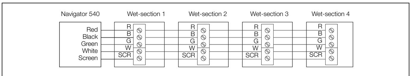
Fig. B.2 Serial connections
