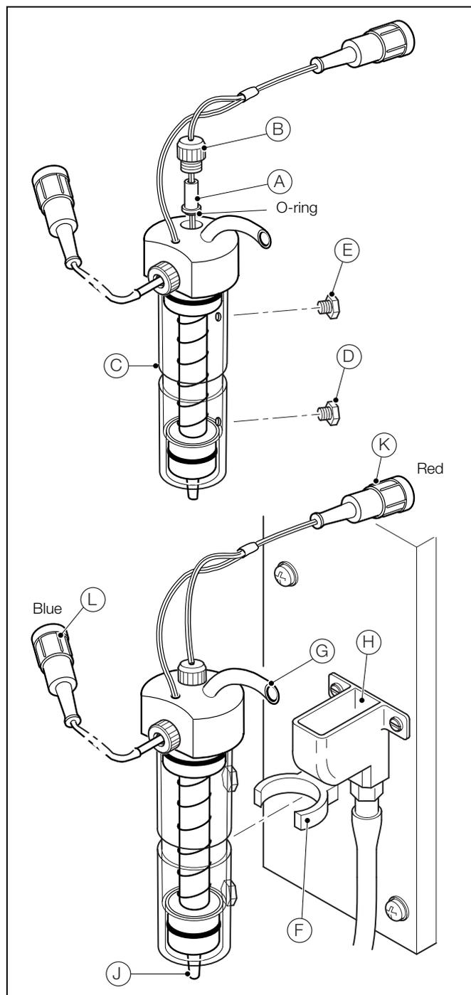
Fig. 8.6 Hydrazine sensor reassembly and fitting
