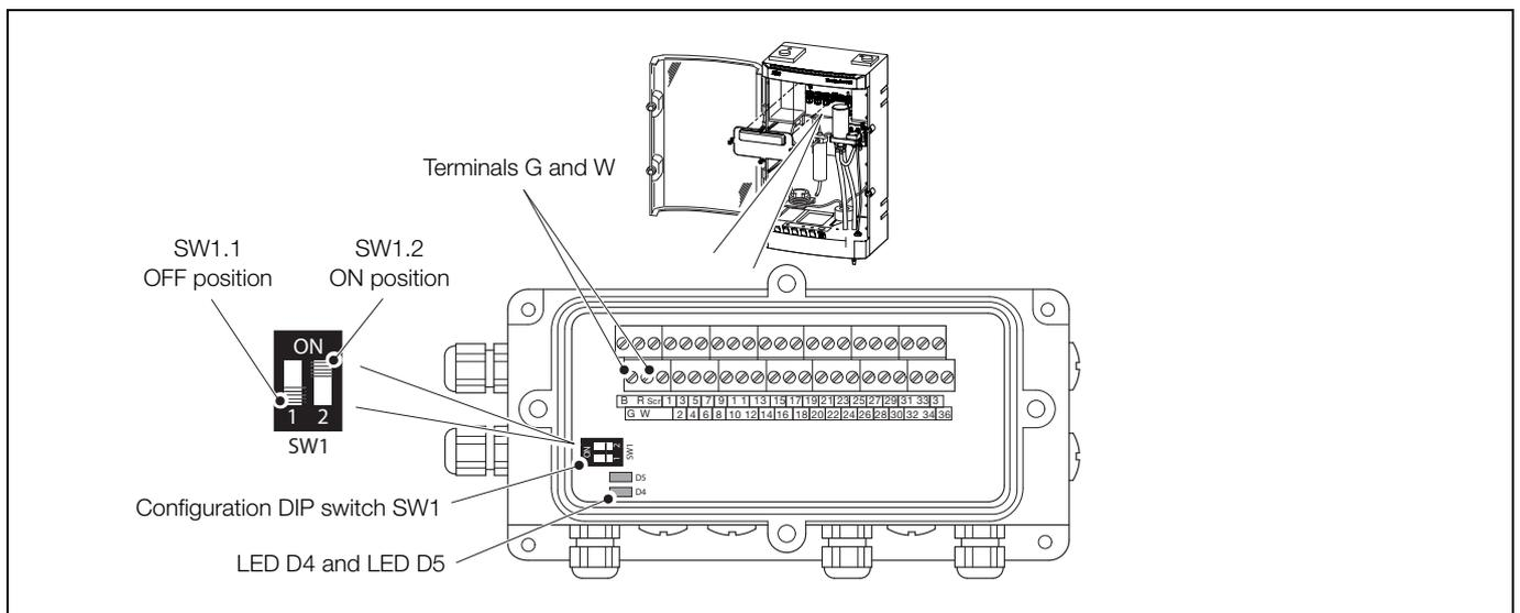
Fig. B.1 Configuration DIP switch SW1 and LED D4 / D5 location
