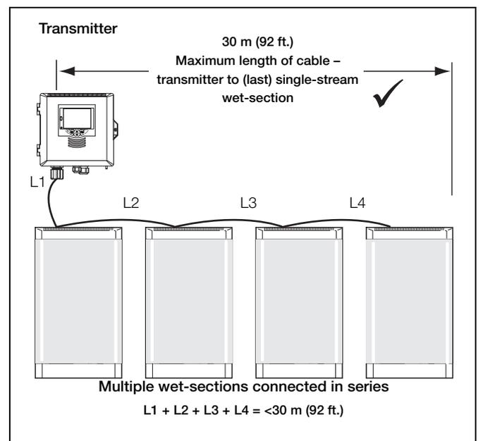
Fig. 3.10 Multiple wet-section setup - maximum cable length
