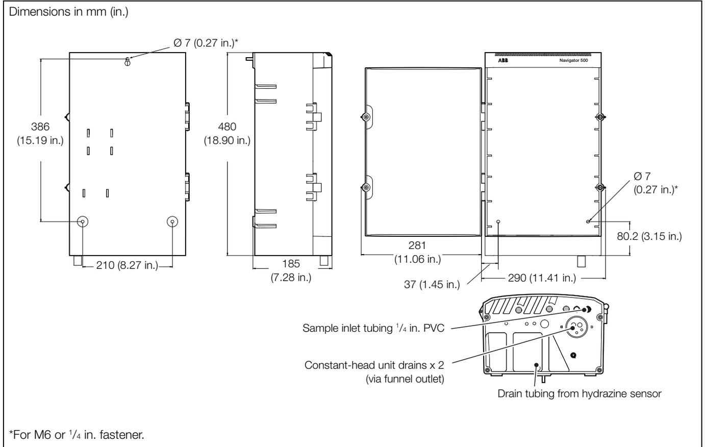
Fig. 3.2 Hydrazine wet-section dimensions
