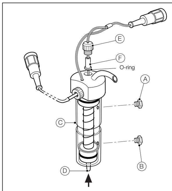
Fig. 8.5 Hydrazine sensor dismantling
