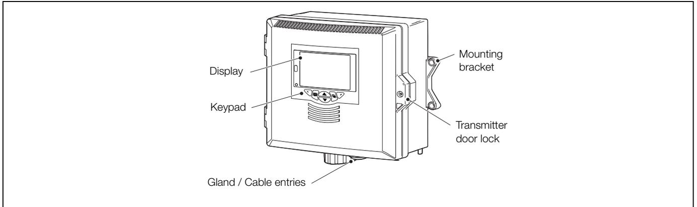
Fig. 2.2 Navigator 540 transmitter – main components
