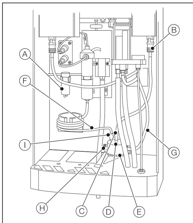
Fig. 8.2 Replacing the microporous disc
