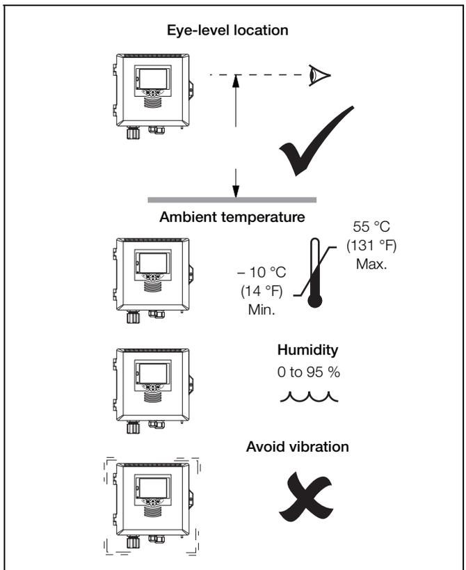
Fig. 3.6 Transmitter location
