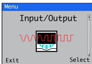
*Input/Output* level enables configuration of analog outputs, digital inputs and outputs and relays.
