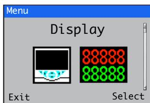
Used to select the display language, setup *Operator* page templates (1 to 5), enable diagnostic, view and log functions, set the device's display brightness / contrast and set the time and date.
