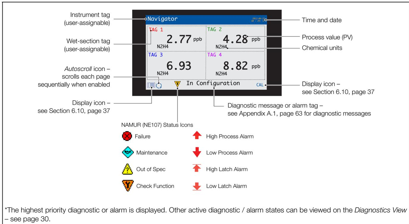
Fig. 6.4 Operator Page 1 (hydrazine multiple wet-section)
