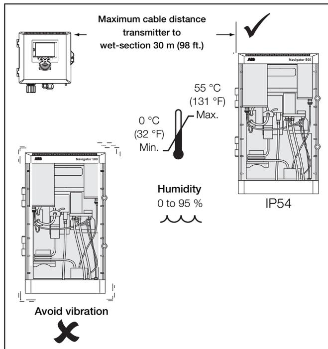
Fig. 3.1 Locating the wet-section
