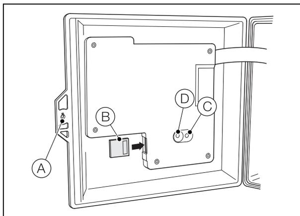
Fig. 6.12 SD card / USB stick insertion and removal
