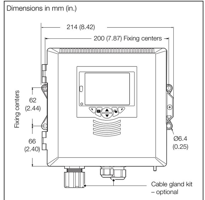
Fig. 3.9 Transmitter wall-mount option
