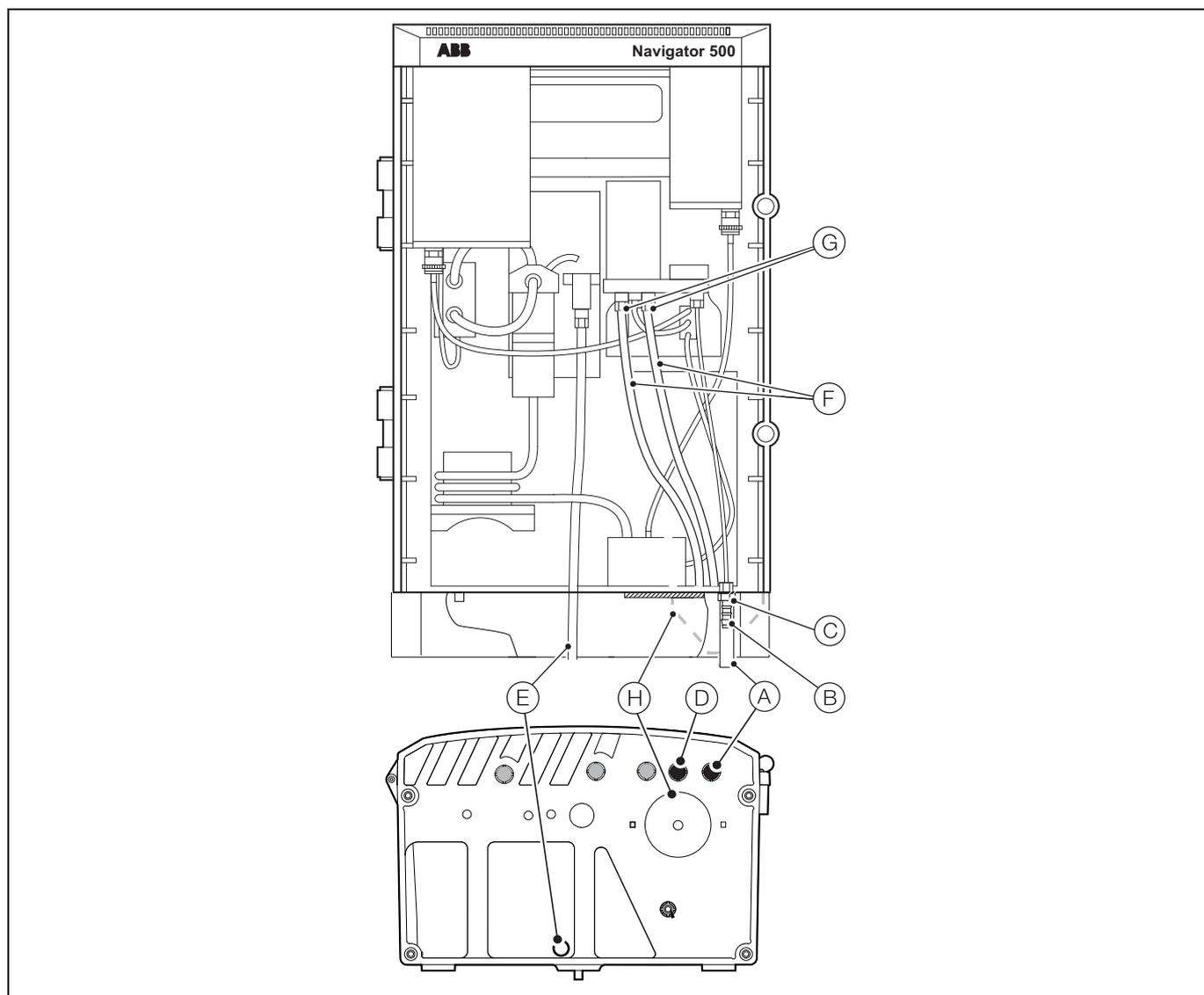
Fig. 3.4 Connecting the external sample lines and drains
