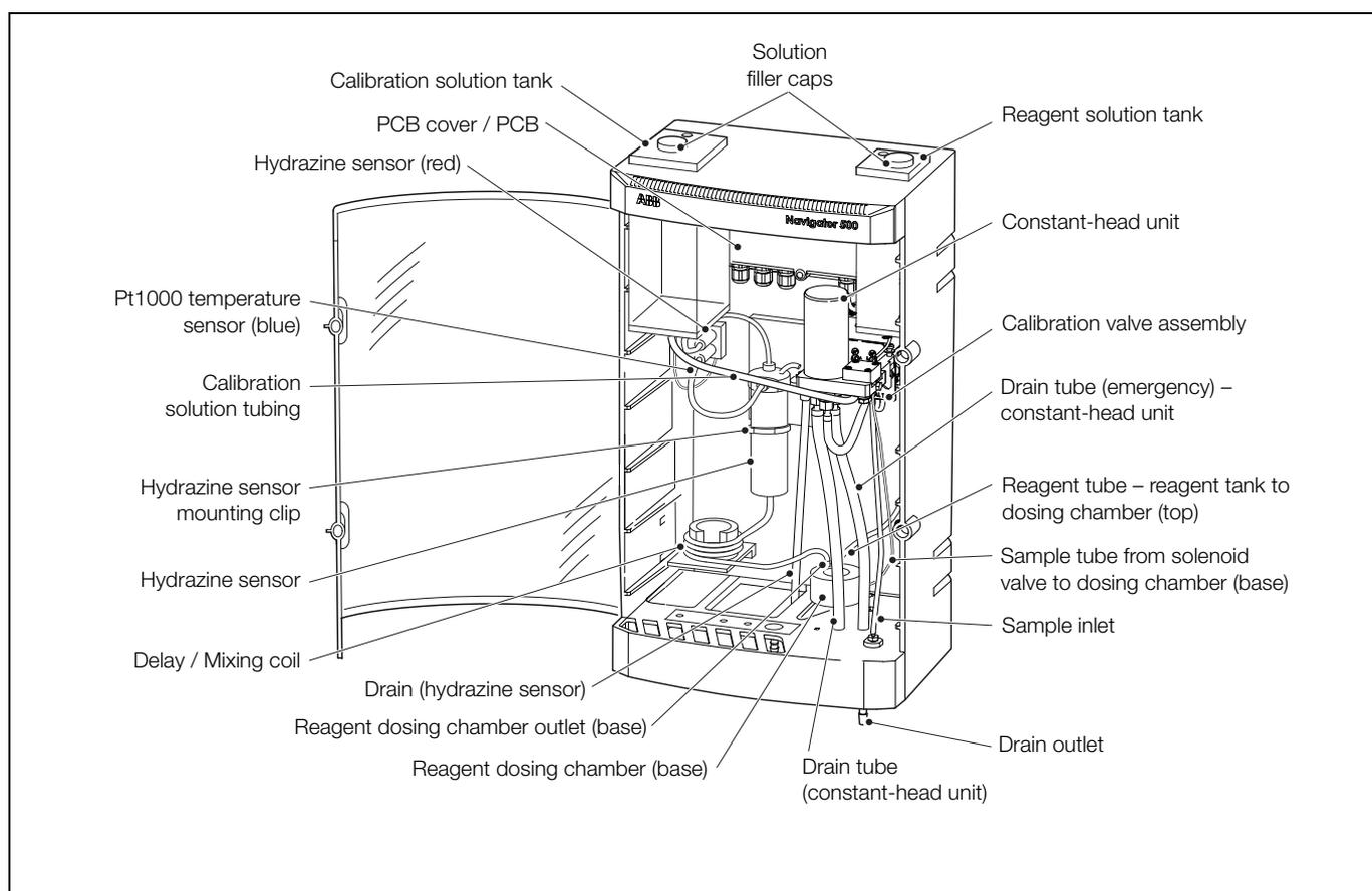
Fig. 2.1 Navigator 550 hydrazine wet-section – main components
