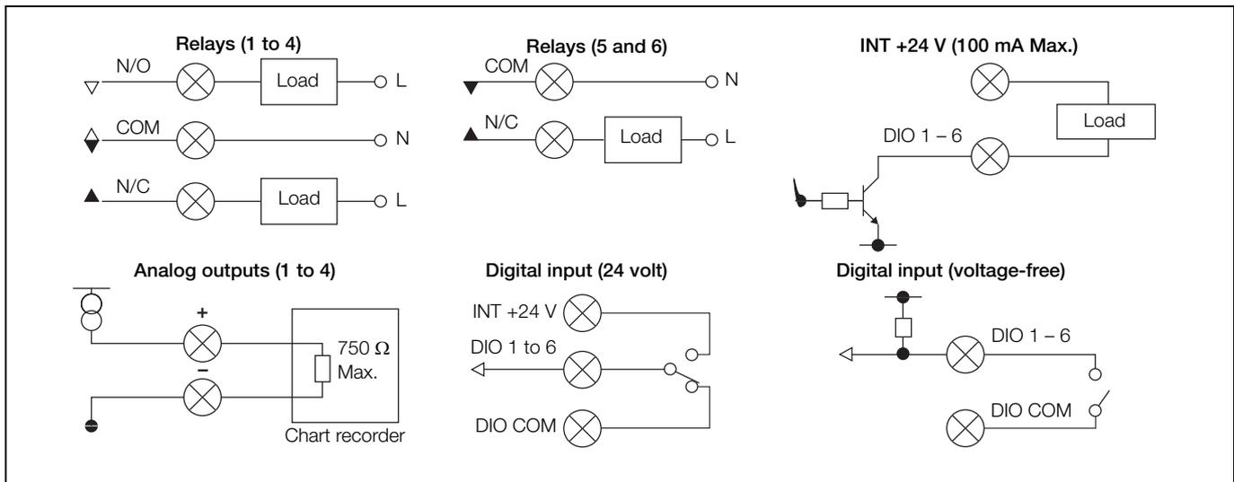
Fig. 3.15 Digital I/O, relays and analog output connections
