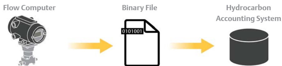
Figure 6. Synchronizing the accounting system with the flow computer database.
