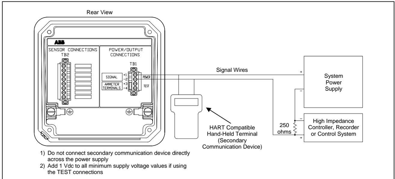
Figure 3-1 Analog Mode Wiring Diagram
