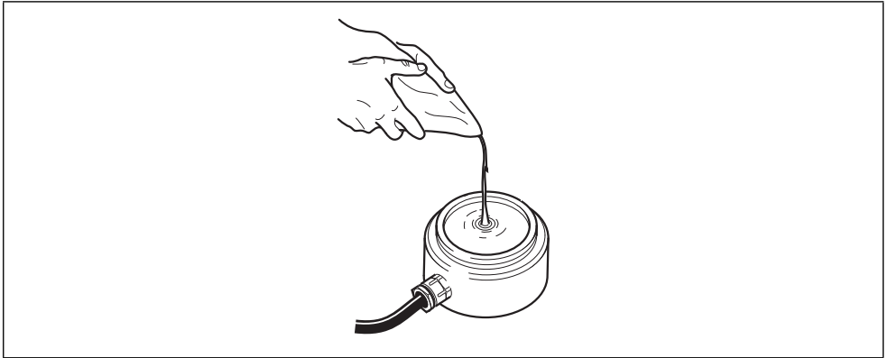
Fig. 3.3 Potting the sensor terminal box
