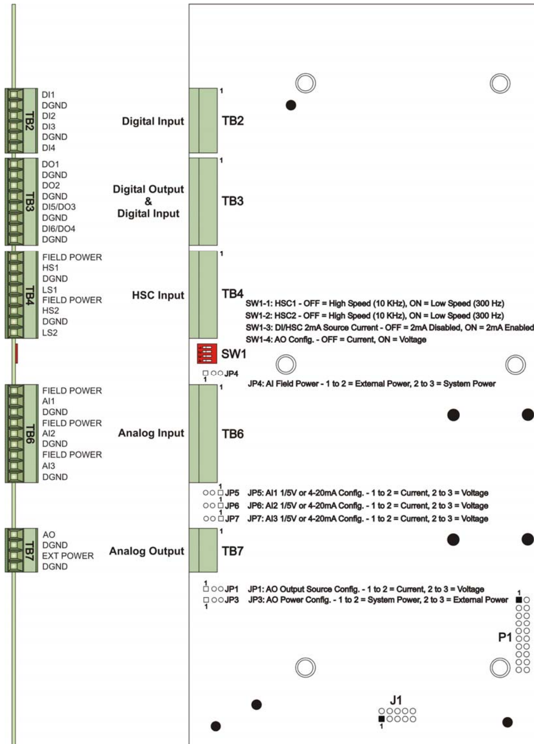
Figure 3-1. Process I/O Board Component Identification Diagram
