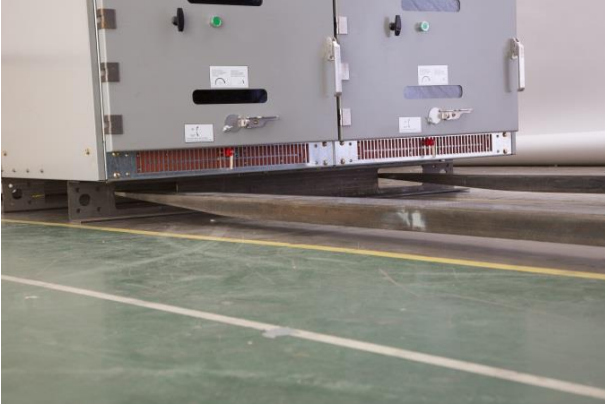
Figure 3: Forklift forks penetrating shipping channels
