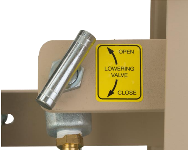
Figure 19: Lift truck control valve
