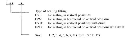
The constructional characteristics and the identification of the different types of sealing fittings are reported in the documents annexed to this certificate.
