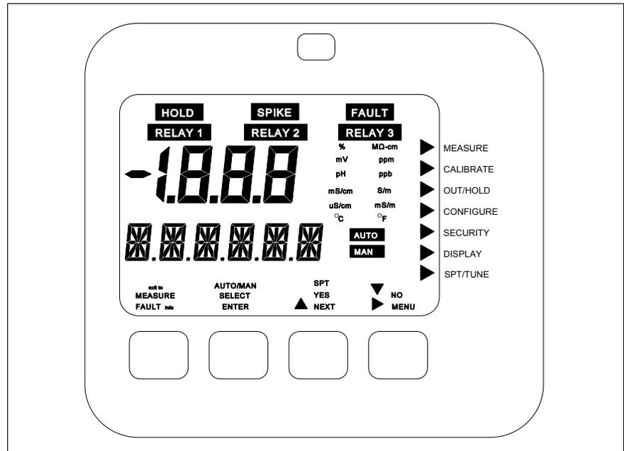
Figure 4-1. Fully Energized Display And Supporting Information. The top set of icons informs the user of an abnormal operating condition such as an output HOLD condition, FAULT condition, diagnostic SPIKE output, or RELAY activation. These icons are only energized when such a condition is detected and are active in all modes of operation.
