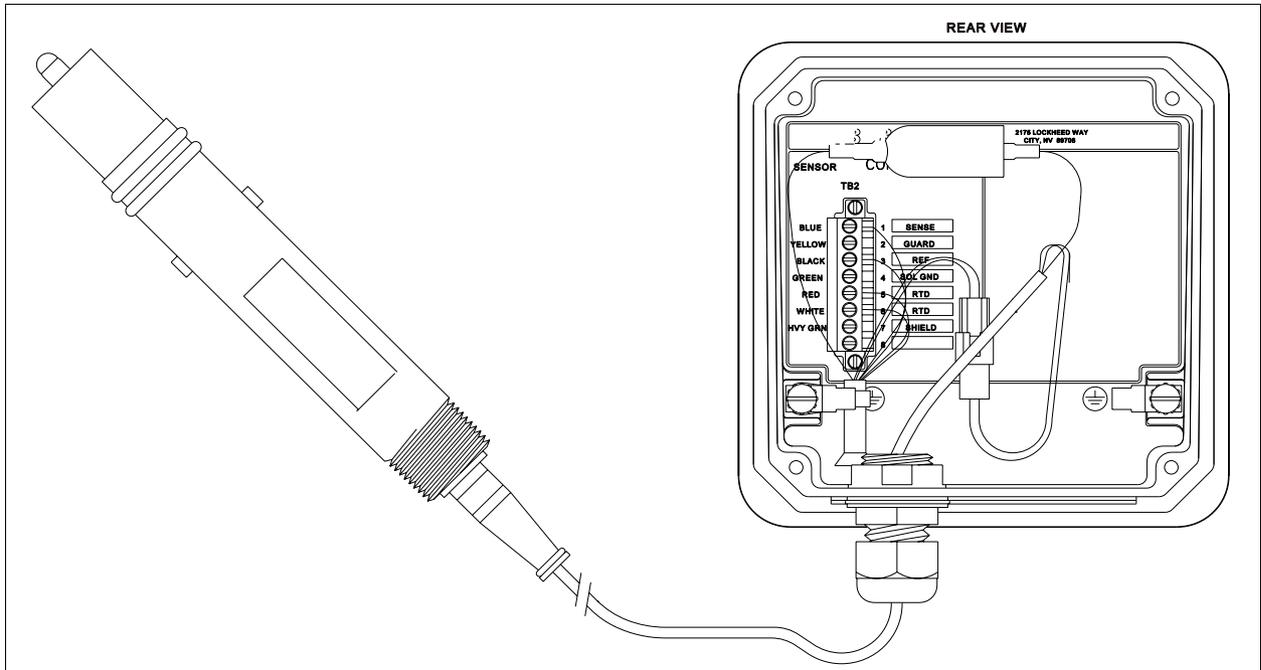
Figure 3-8. BNC Adapter Installation and Wiring Diagram
