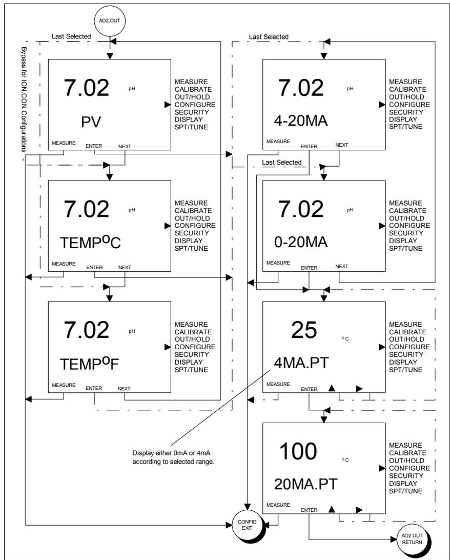
Figure 8-7. Screen Flow Diagram For Analog Output Two Configure State of Operation.
