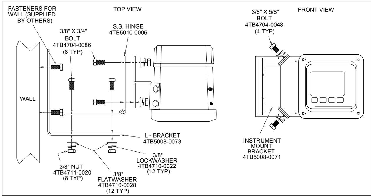
Figure 3-3. Hinge Mount Installation Diagram
