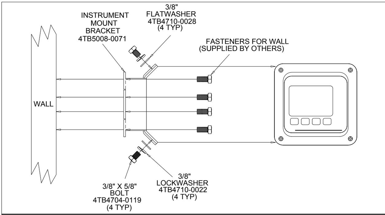
Figure 3-4. Wall Mount Installation Diagram
