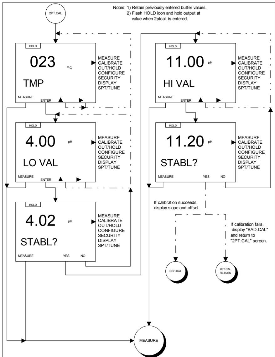
Figure 6-3. Screen Flow Diagram For Two-Point Process Calibration.
