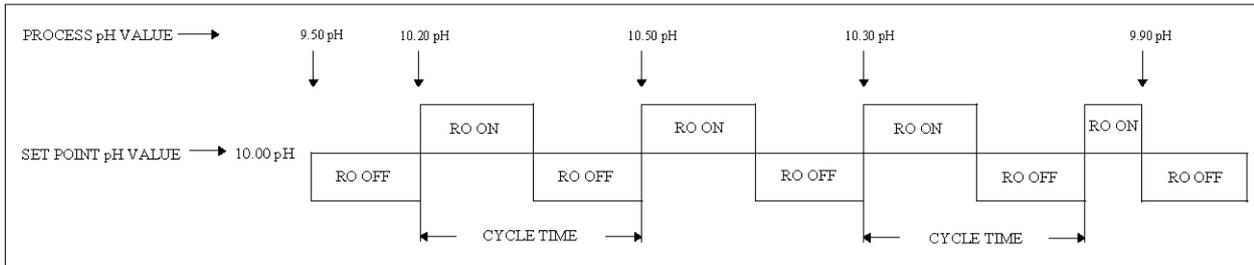
Figure 2.2. Cycle Timer High Set Point Example.
