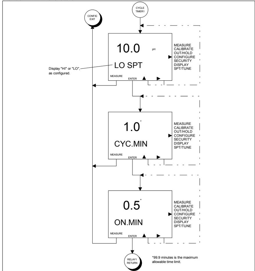
Figure 8-13. Screen Flow Diagram For Setting the Cycle Timer Relay Output Configure State Set the Cycle Timer parameters of a Relay Output using Figure 8-13 as reference and the following procedure:
