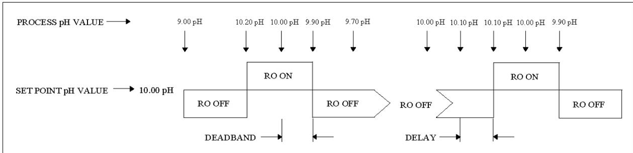
Figure 2-1. High Set Point and Time Delay Example.
