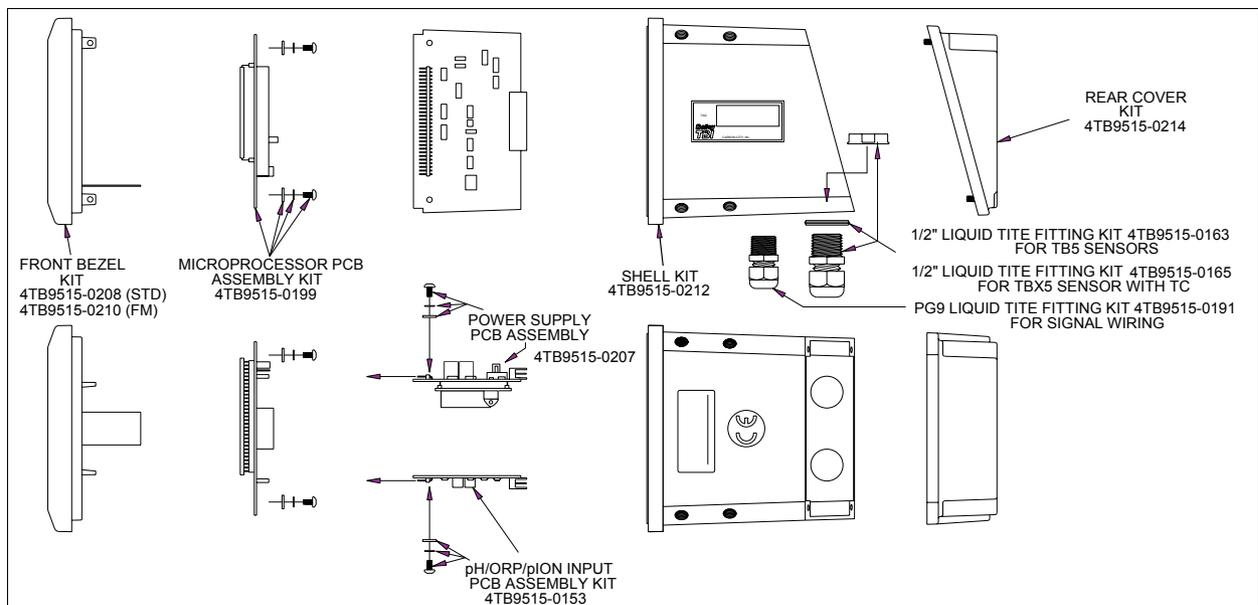
Figure 16-1. TB84PH Advantage Series Exploded View Showing Kit Assignments.
