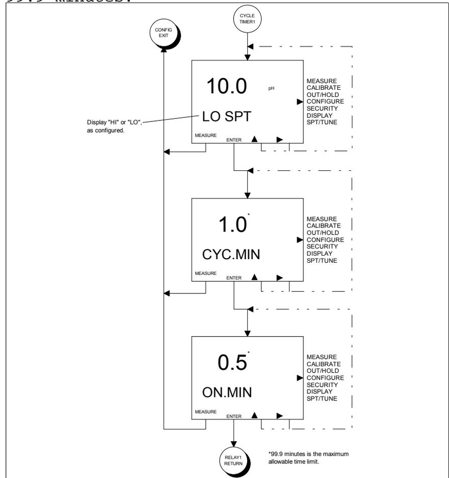
Figure 8-13. Screen Flow Diagram For Setting the Cycle Timer Relay Output Configure State of Operation. Set the Cycle Timer parameters of a Relay Output using Figure 8-13 as reference and the following procedure:
