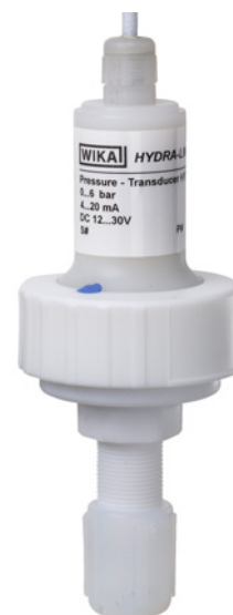
HYDRA-line Model HD, transducer 4 ... 20 mA, 2-wire system and dead-end 1/2" flare process connection
