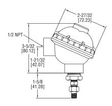
The **MODEL A-709** Temperature Enclosure can be used to mount our Series 651 and 659 transmitters to any of our 1/4" diameter temperature sensors. The screw on enclosure core can be quickly removed and has a chain to prevent it from getting lost. The Model A-709 comes with the necessary adapters and fittings for attaching the temperature sensor.
