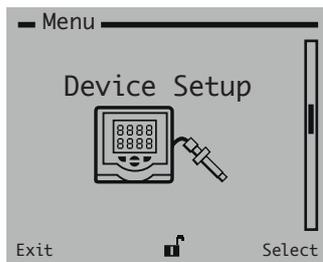
Used to setup security parameters, set PDM compatibility (for HART-enable transmitters) and to reset default (factory-set) parameters.
