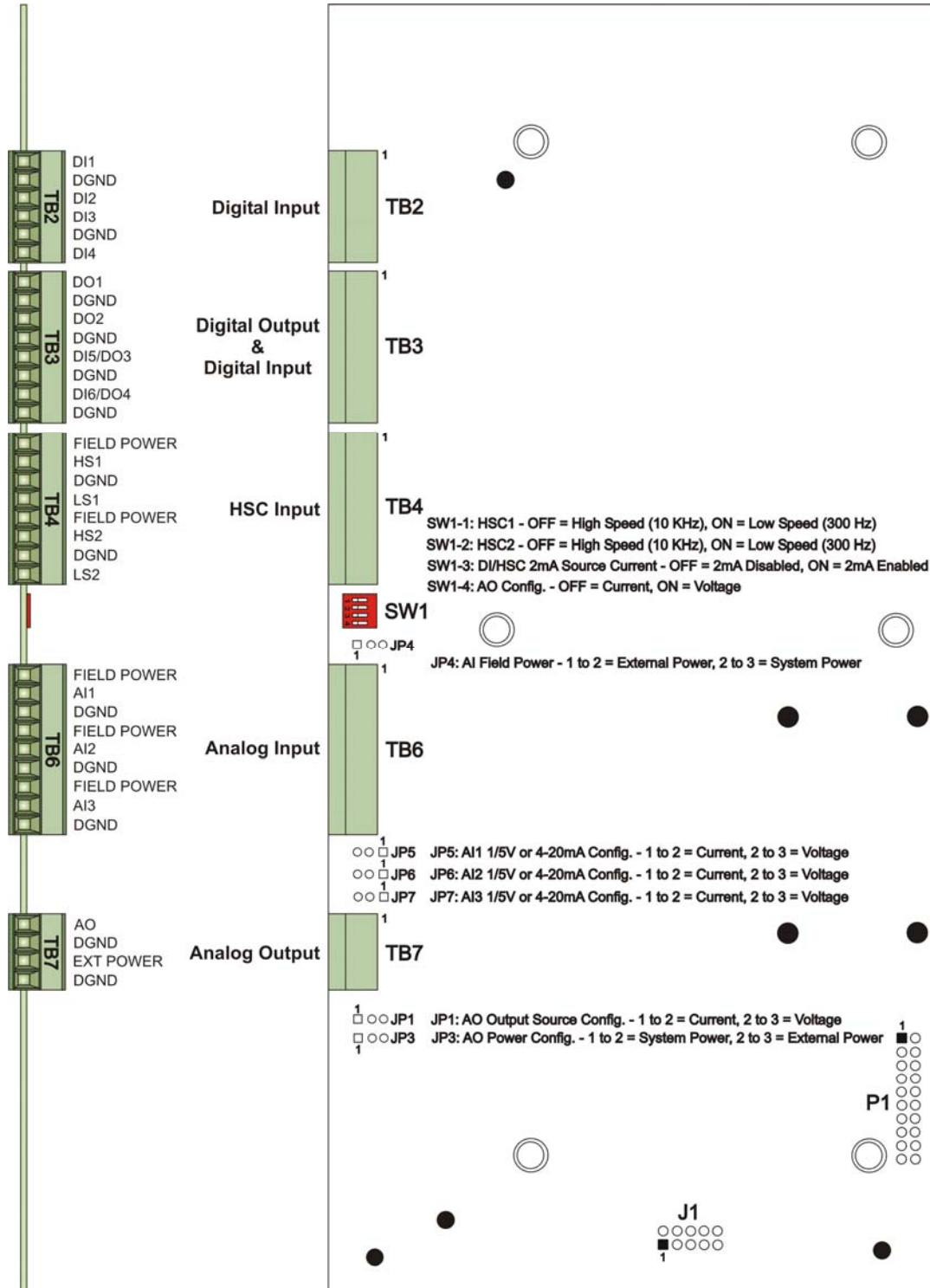
Figure 3-1. Process I/O Board Component Identification Diagram
